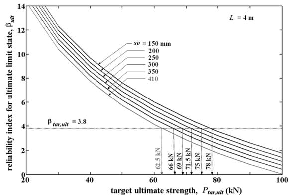
Fig. 13 Target ultimate load-reliability index curves at various widths of the web opening for the governed failure mode
