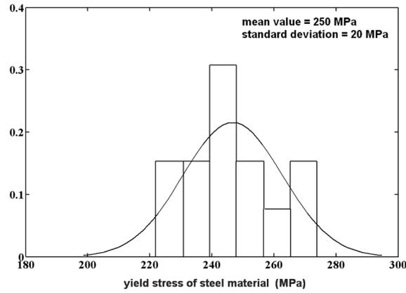
Fig. 6 Histogram and density curve for the yield stresses of the steel material
