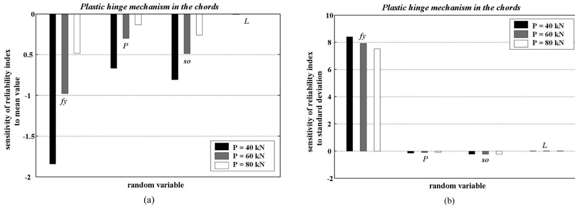
Fig. 17 Sensitivity of the reliability index to (a) the mean value and (b) the standard deviation of random variables for the governed failure mode
