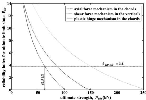
Fig. 12 Ultimate load-reliability index curves for possible failure mechanisms
