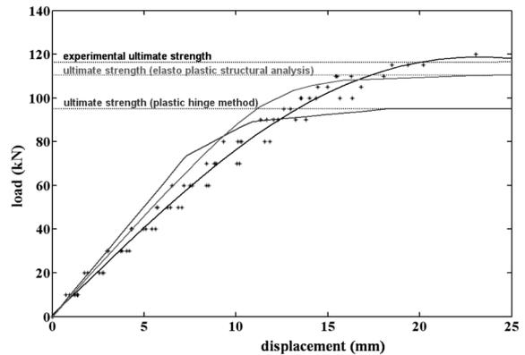
Fig. 8 Load-displacement curves
