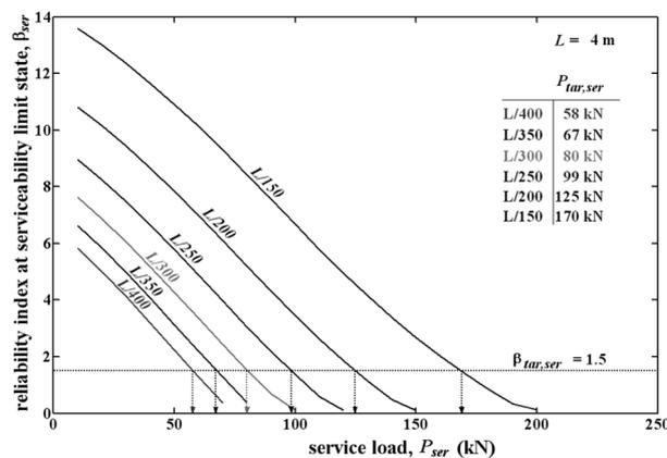
Fig. 15 Service load-reliability index curves for various deflection limits
