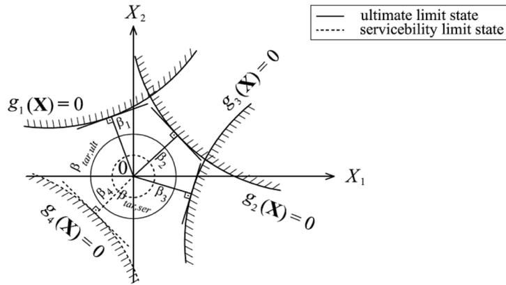
Fig. 1 Reliability indices for multiple performance functions in the standard normal space
