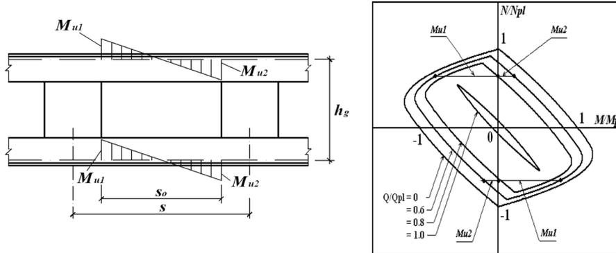
Fig. 11 Plastic hinge mechanism and interaction curves for the chords
