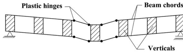
Fig. 9 Failure mechanism of the tested beams and configuration of the plastic hinges
