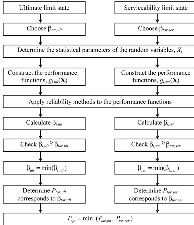
Fig. 2 Flow chart for the proposed algorithm
