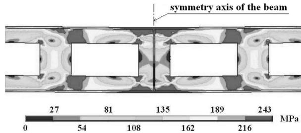
Fig. 10 Elasto plastic stress distributions at the middle part of the beam
