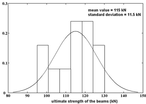
Fig. 7 Histogram and density curve for ultimate strengths of the beams
