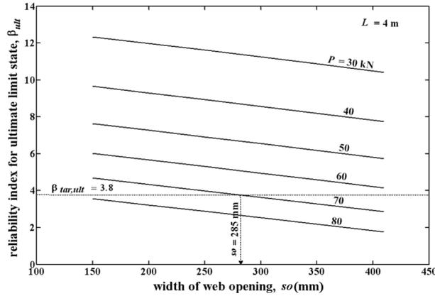
Fig. 14 Width of the web opening-reliability index curves for various beam loads
