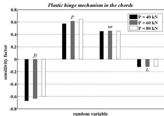
Fig. 16 Sensitivity factors of random variables for the governed failure mode
