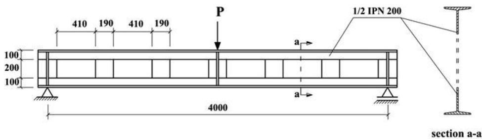
Fig. 3 Geometry and loading of the tested beams (in mm)
