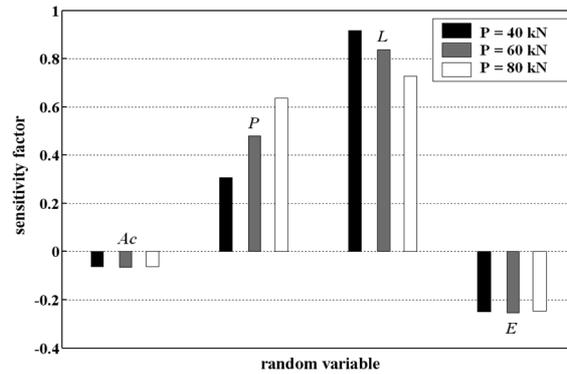
Fig. 18 Sensitivity factors of random variables for a deflection limit of  $L/300$
