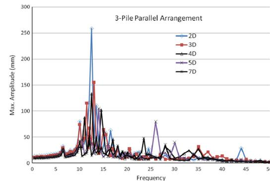
Fig. 7 Frequency-amplitude curve for 3-pile in parallel configuration
