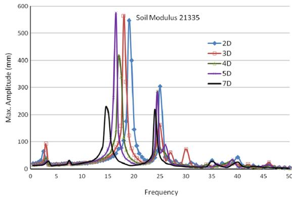
Fig. 8 Frequency-amplitude curve for soil modulus 21335 kN/m<sup>2</sup>
