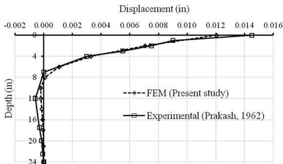
Fig. 2(a) Comparison of displacement of pile
