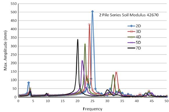
Fig. 9 Frequency-amplitude curve for soil modulus 42670 kN/m<sup>2</sup>
