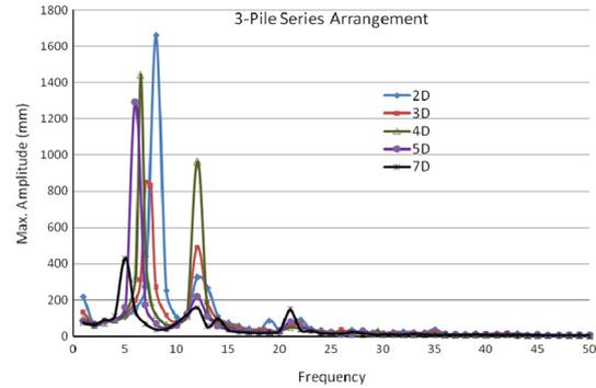
Fig. 5 Frequency-amplitude curve for 3-pile in series configuration
