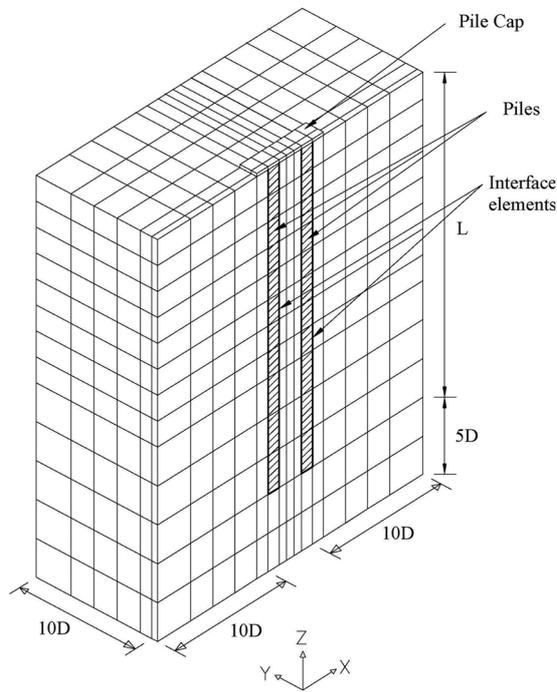
Fig. 1(b) Typical discretization scheme for two piles in series arrangement
