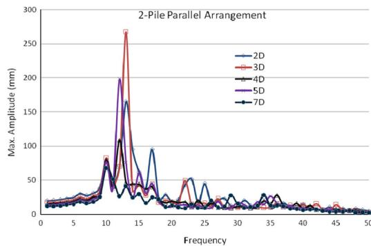
Fig. 6 Frequency-amplitude curve for 2-pile in parallel configuration
