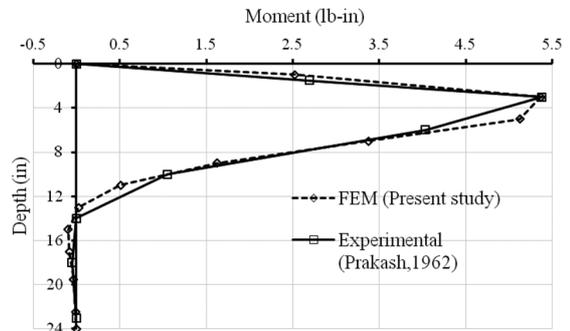
Fig. 2(b) Comparison of B.M. distribution in pile
