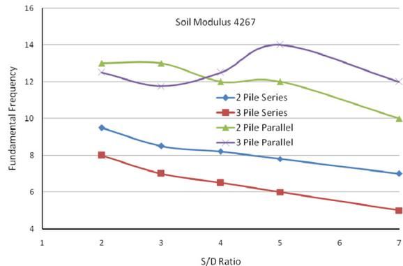
Fig. 10 Comparison of response for different pile configurations
