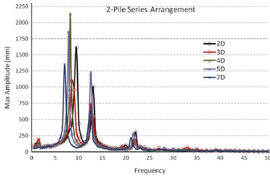
Fig. 4 Frequency-amplitude curve for 2-pile series
