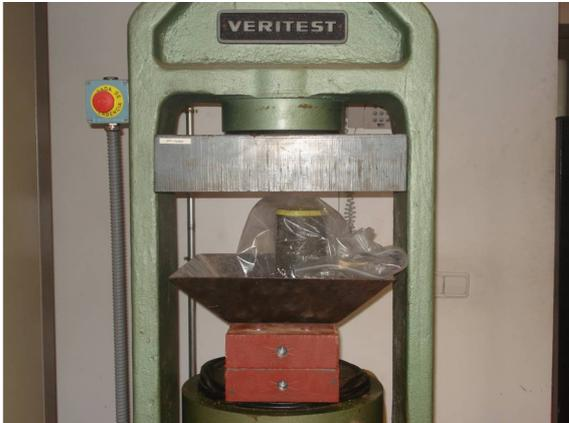
Fig. 3 Compression test
