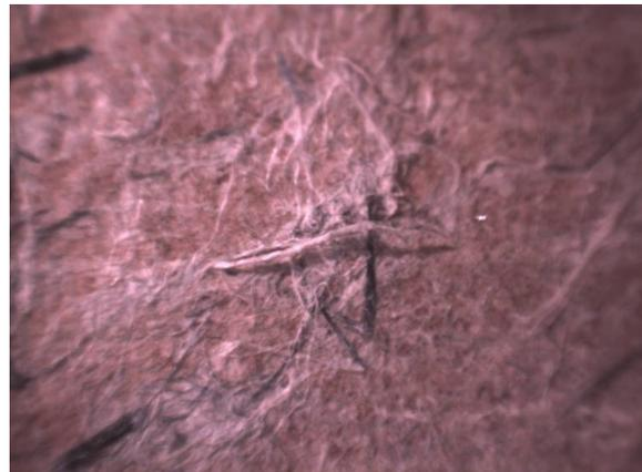
Fig. 10. Microscopy image of pipe's inner surface (weak pipe)
