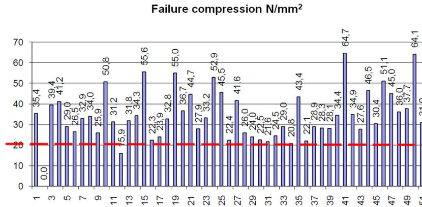
Fig. 8. Bar chart of failure stresses by compression test
