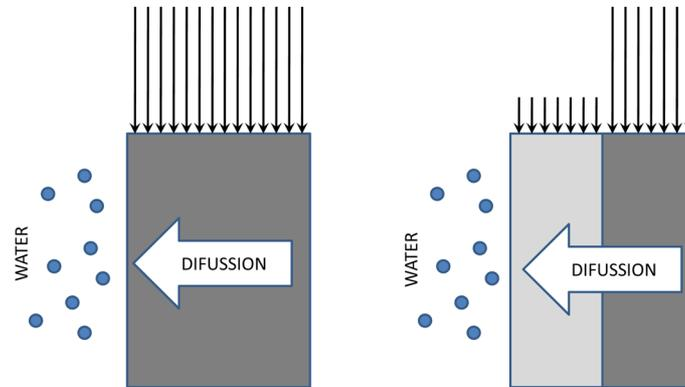
Fig. 13 Leaching mechanism of loss of strength
