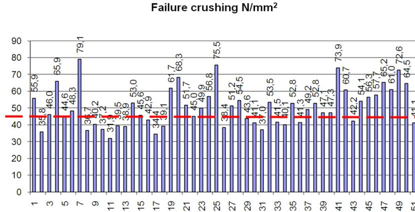
Fig. 6 Bar chart of failure stresses by crushing test
