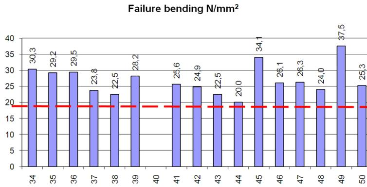
Fig. 7. Bar chart of failure stresses by bending test
