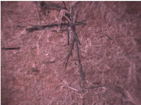
Fig. 9 Microscopy image of pipe's inner surface (weak pipe)
