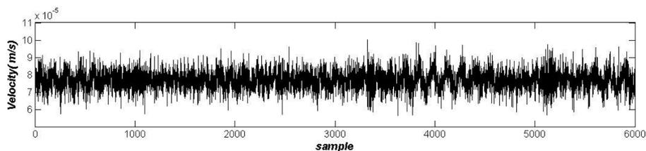
Fig. 7 One of the records of the building at the mass center of second floor
