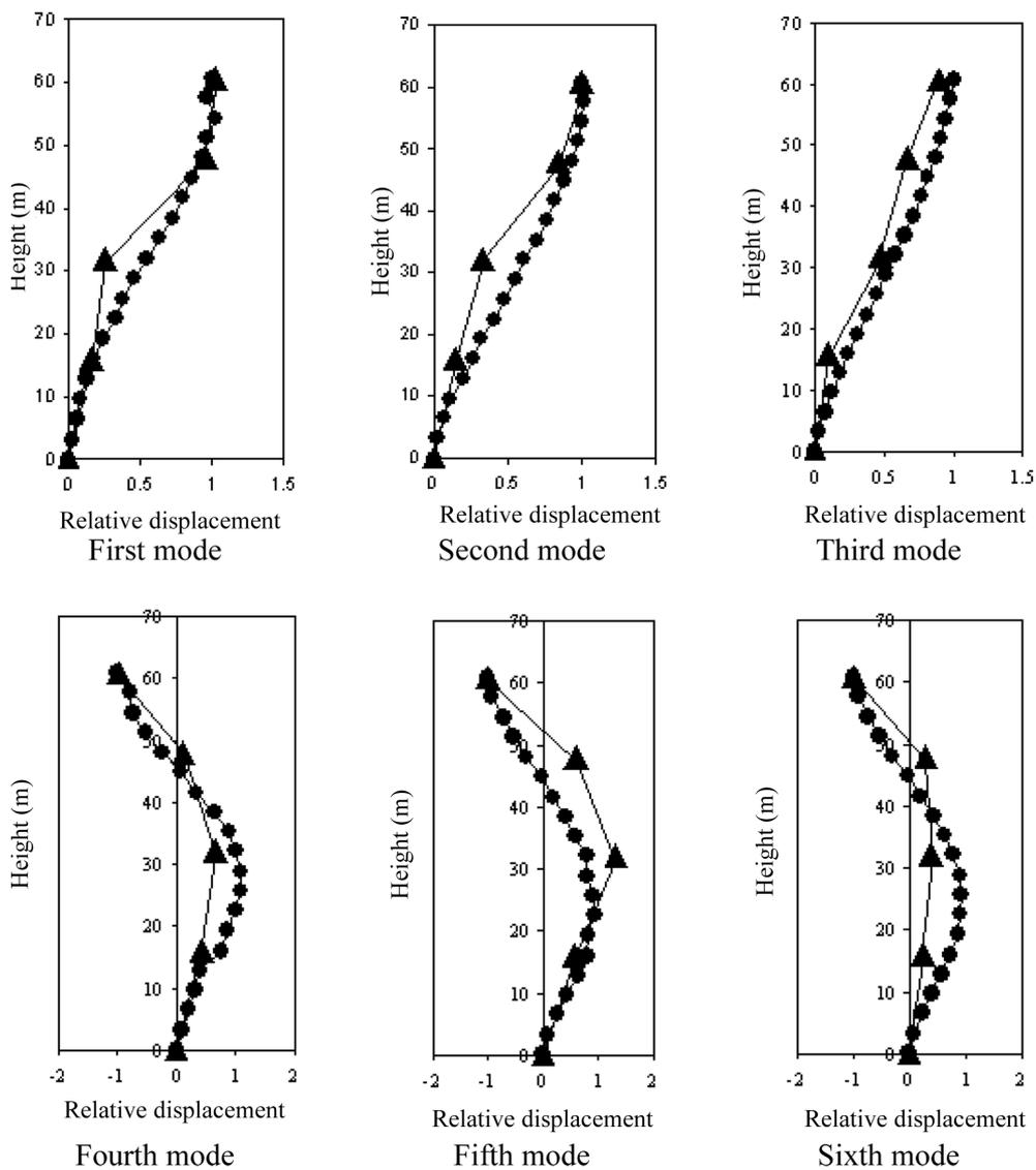
Fig. 11 Mode shapes obtained from finite element model and ambient vibration tests (▲: Tests results, \* : Model results)
