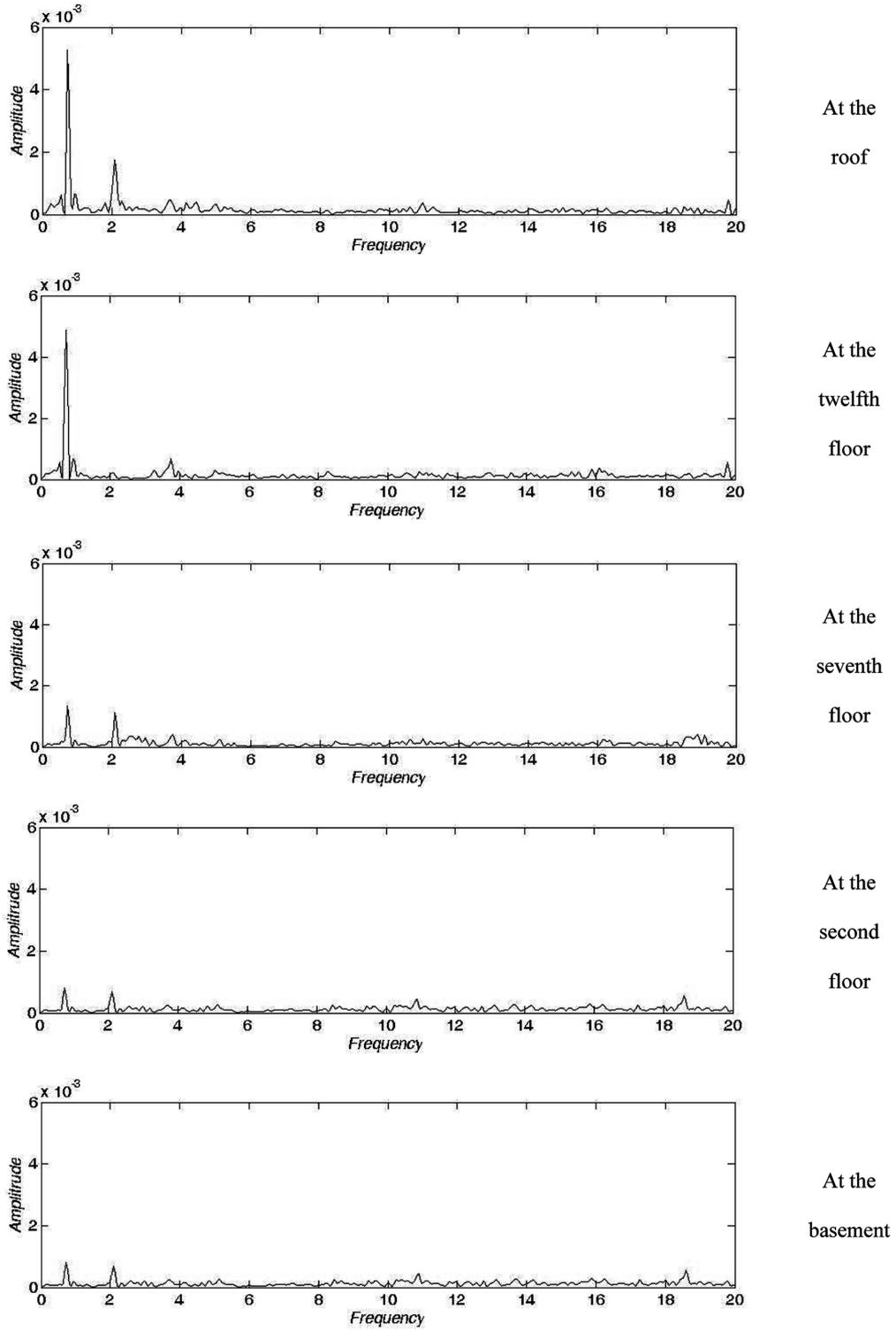
Fig. 9 Translational Fourier amplitude spectra at various floors of the building
