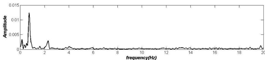
Fig. 8 One of the Fourier amplitude spectra corresponding to a record at the roof of the building
