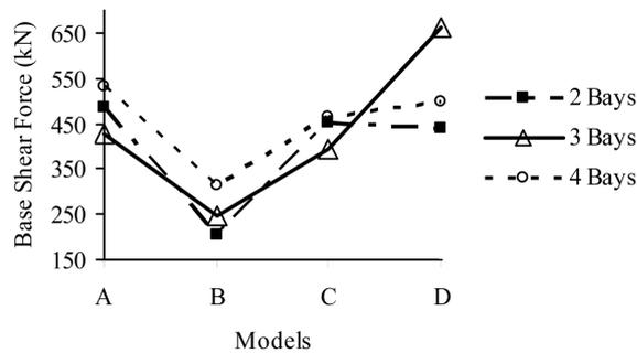
Fig. 5 The maximum base shear force for  $(H/B) = 1$
