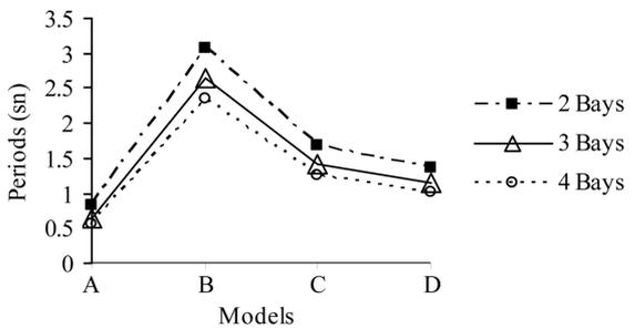
Fig. 11 Structure period for (H/B) = 2
