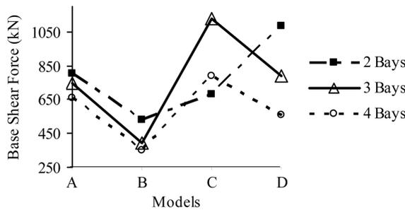
Fig. 9 The maximum base shear force for (H/B) = 2
