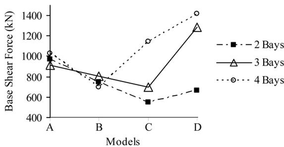
Fig. 13 The maximum base shear force for (H/B) = 3
