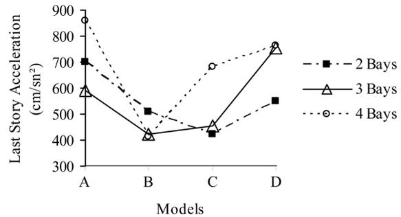
Fig. 16 The maximum last storey acceleration for  $(H/B) = 3$
