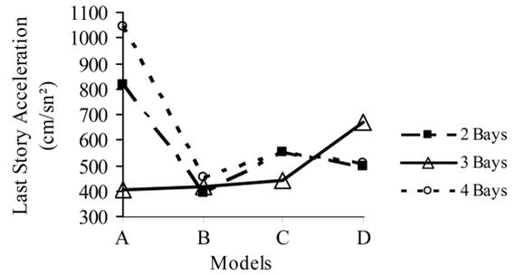
Fig. 8 The maximum last storey acceleration for (H/B) = 1
