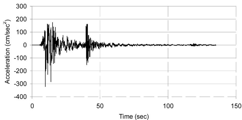
Fig. 4 The records of 17 August 1999 Marmara Earthquake Yarimca-Petkim N-S acceleration component
