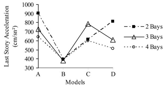
Fig. 12 The maximum last storey acceleration for (H/B) = 2
