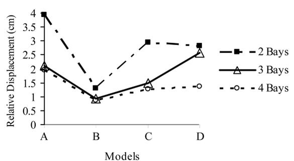
Fig. 6 The maximum relative displacement for  $(H/B) = 1$
