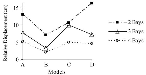
Fig. 10 The maximum relative displacement for (H/B) = 2
