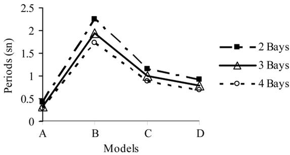
Fig. 7 Structure period for (H/B) = 1
