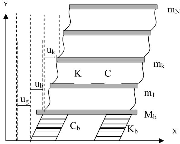
Fig. 2 Mathematical model of multi-storey structures in which base is isolated
