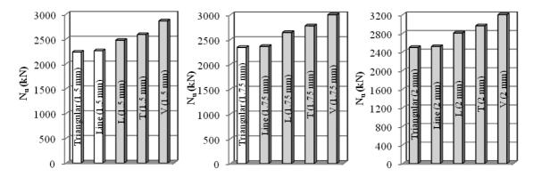
Fig. 27 Effect of shape of steel sheeting stiffeners on ultimate axial load capacity of the columns (2 on side stiffeners)
