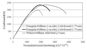
Fig. 20 Axial load-normalized axial shortening plots for columns with different number of Triangular stiffeners (cold-formed 1.75 mm) and without stiffener (mild steel 2.5 mm)
