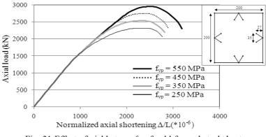
Fig. 31 Effect of yield stress  $f_{yp}$  of cold-formed steel sheet
