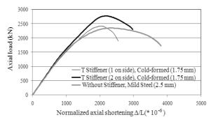
Fig. 17 Axial load-normalized axial shortening plots for columns with different number of T stiffeners (cold-formed 1.75 mm) and without stiffener (mild steel 2.5 mm)
