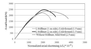
Fig. 13 Axial load-normalized axial shortening plots for columns with different number of L stiffeners (cold-formed 1.5 mm) and without stiffener (mild steel 2.5 mm)
