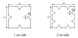
Fig. 10 Cross sections of the concrete-filled steel composite columns (Triangular stiffeners & cold-formed steel sheets of 1.5, 1.75 & 2 mm)
