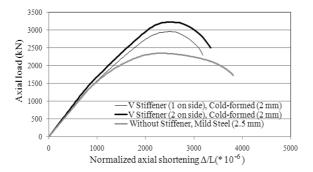
Fig. 21 Axial load-normalized axial shortening plots for columns with different number of V stiffeners (cold-formed 2 mm) and without stiffener (mild steel 2.5 mm)
