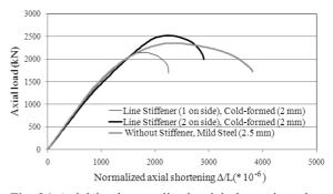
Fig. 24 Axial load-normalized axial shortening plots for columns with different number of Line stiffeners (cold-formed 2 mm) and without stiffener (mild steel 2.5 mm)
