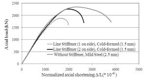
Fig. 14 Axial load-normalized axial shortening plots for columns with different number of Line stiffeners (cold-formed 1.5 mm) and without stiffener (mild steel 2.5 mm)
