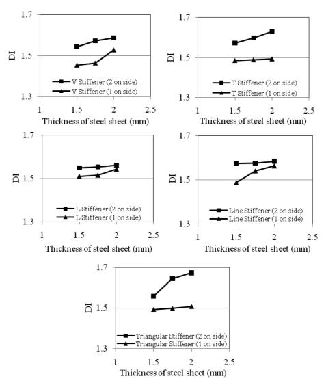
Fig. 28 Effects of stiffeners and thickness of steel sheet on ductility of the columns
