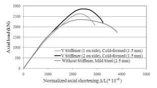
Fig. 11 Axial load-normalized axial shortening plots for columns with different number of V stiffeners (cold-formed 1.5 mm) and without stiffener (mild steel 2.5 mm)
