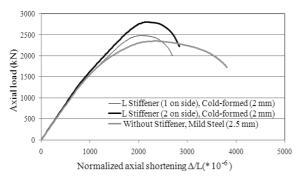
Fig. 23 Axial load-normalized axial shortening plots for columns with different number of L stiffeners (cold-formed 2 mm) and without stiffener (mild steel 2.5 mm)
