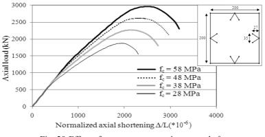
Fig. 29 Effect of concrete compressive strength  $f_c$
