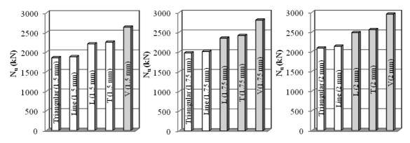
Fig. 26 Effect of shape of steel sheeting stiffeners on ultimate axial load capacity of the columns (1 on side stiffeners)
