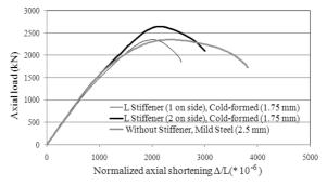
Fig. 18 Axial load-normalized axial shortening plots for columns with different number of L stiffeners (cold-formed 1.75 mm) and without stiffener (mild steel 2.5 mm)
