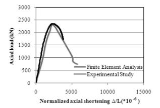
Fig. 5 Axial load-normalized axial shortening curves of the concrete-filled steel composite column (without stiffener, mild steel)
