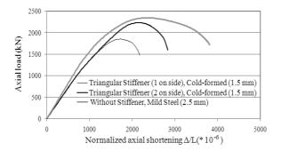
Fig. 15 Axial load-normalized axial shortening plots for columns with different number of Triangular stiffeners (cold-formed 1.5 mm) and without stiffener (mild steel 2.5 mm)
