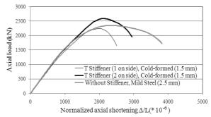
Fig. 12 Axial load-normalized axial shortening plots for columns with different number of T stiffeners (cold-formed 1.5 mm) and without stiffener (mild steel 2.5 mm)
