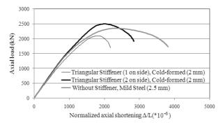
Fig. 25 Axial load-normalized axial shortening plots for columns with different number of Triangular stiffeners (cold-formed 2 mm) and without stiffener (mild steel 2.5 mm)
