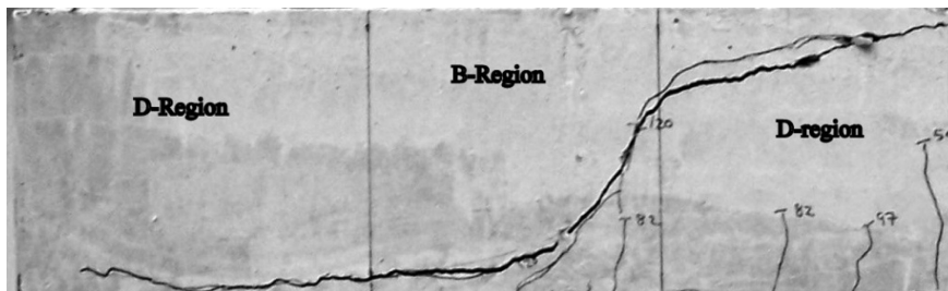
Fig. 7 Cracking pattern of unstrengthened beam
