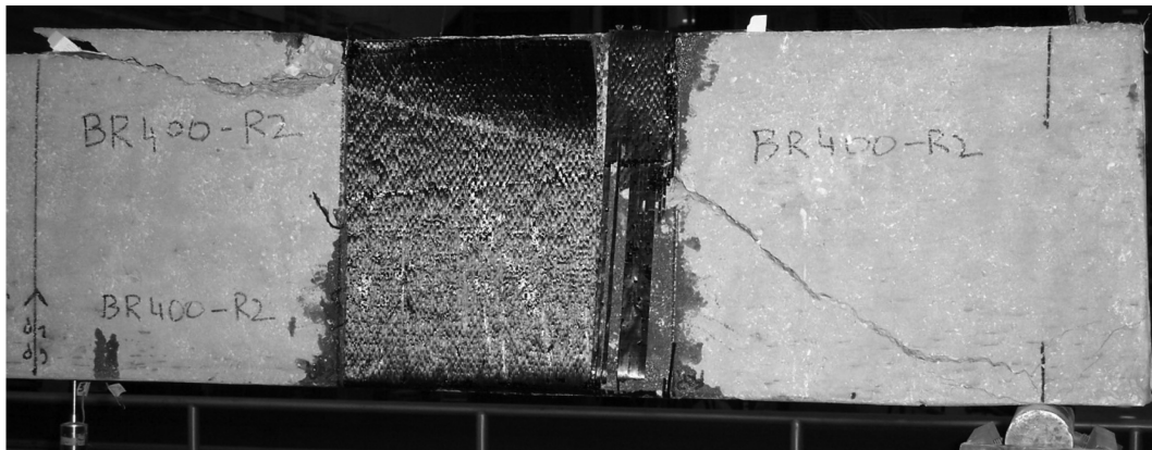
(c) Cracking pattern in beam BR400
