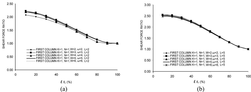
Fig. 5 The effect of variation in band window width on the short column shear force ratio for (a)  $L = 2$  m and (b)  $L = 5$  m
