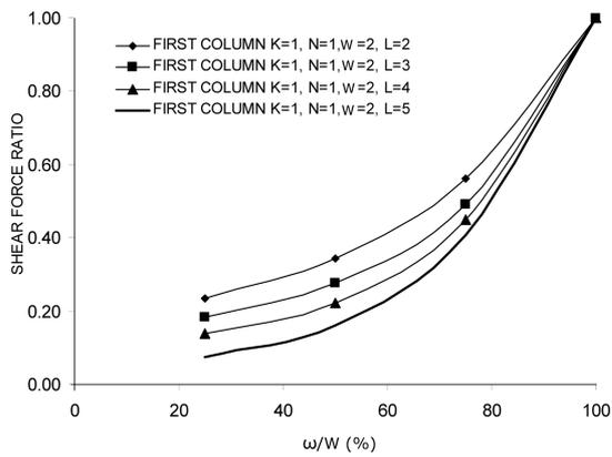
Fig. 8 The effect of band window width on the shear force for  $W = 2$  m
