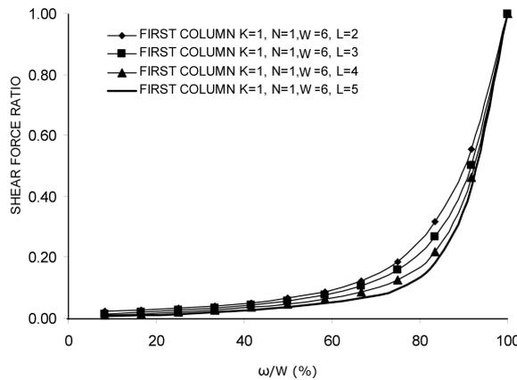
Fig. 10 The effect of band window width on the shear force for  $W = 6$  m
