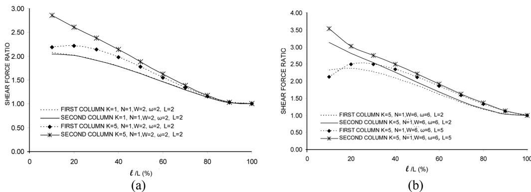
Fig. 7 (a) Variation in the shear force ratios in the 1<sup>st</sup> and 2<sup>nd</sup> columns depending on the increase in the number of stories (b) Variation in the shear force ratios in the 1<sup>st</sup> and 2<sup>nd</sup> columns depending on the variations in the frame width in a 5-storey building
