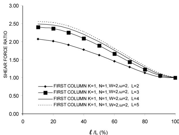
Fig. 4 The variation of short column shear force ratio with storey height ratio
