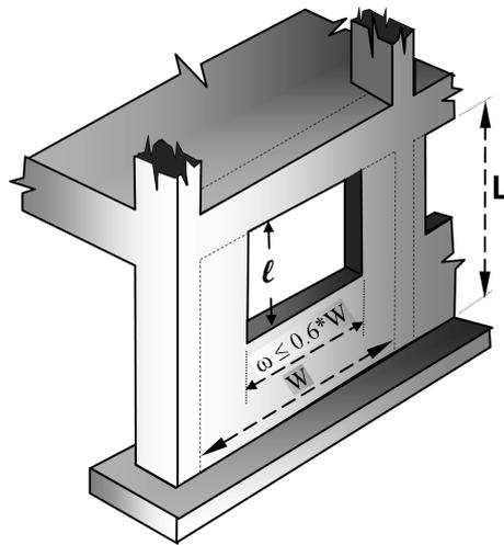
Fig. 11 Band window design in a reinforced concrete frame infill
