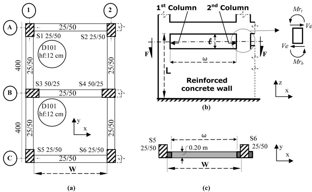
Fig. 3 (a) Plan, (b) the longitudinal section of axis C, (c) cross-section F-F
