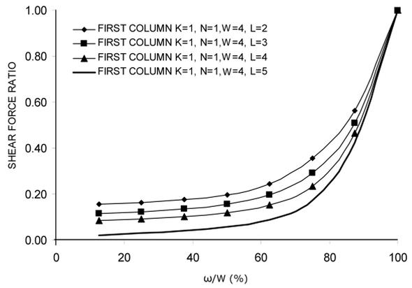
Fig. 9 The effect of band window width on the shear force for  $W = 4$  m
