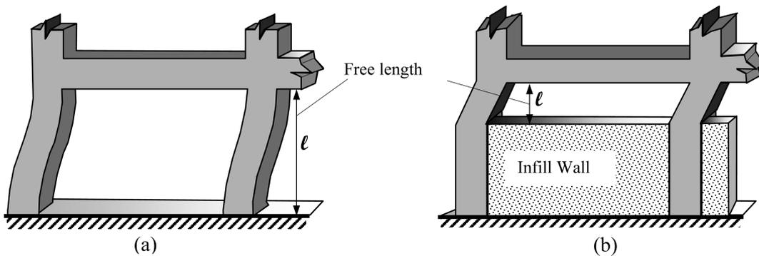
Fig. 2 (a) Freely bending hollow frame, (b) partially infilled frame with shortened column heights
