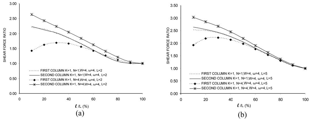
Fig. 6 Variation in the shear force ratios in the 1<sup>st</sup> and 2<sup>nd</sup> columns depending on the increase in the number of bays for (a)  $L = 2$  m and (b)  $L = 5$  m
