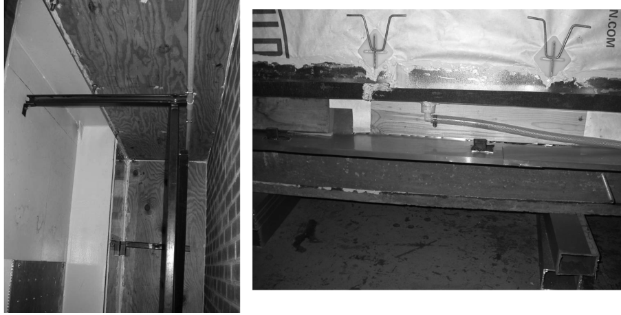
Fig. 8 Water supply at top of the chamber and water collection system behind the BV
