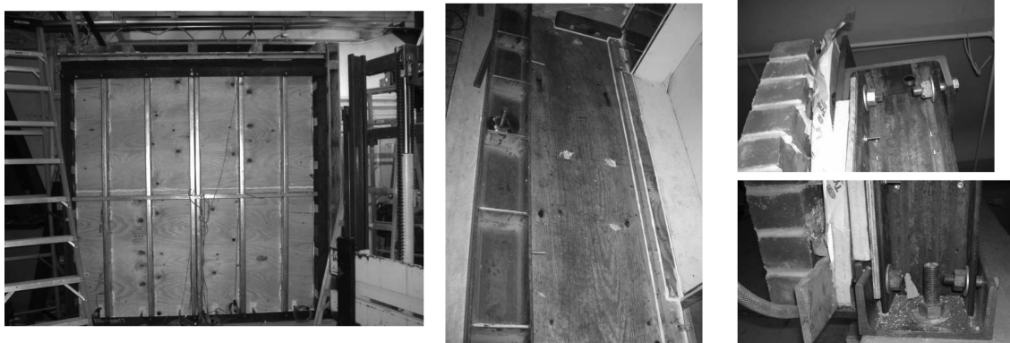
Fig. 3 Backup system, connection details of vertical channels, and stiffeners at bottom channel
