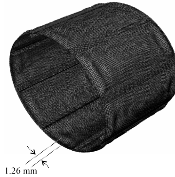
Fig. 10 Quasi static shell deformation with highlighted the radial displacement at 242 kN
