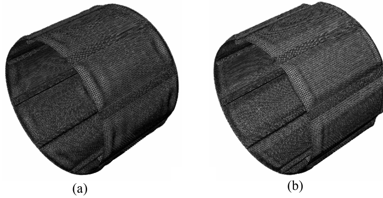
Fig. 12 Comparison of deformed shapes (a) static buckling, (b) dynamic buckling for load step of 200 kN and duration of 0.01 s
