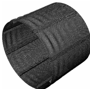
Fig. 3 Buckling shape of the stiffened cylindrical shell
