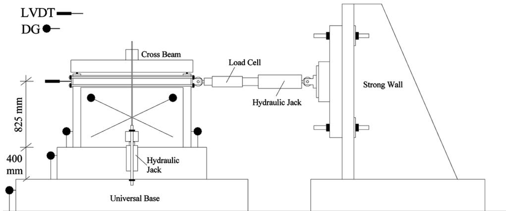
Fig. 8 Details of test set-up, loading system and instrumentation
