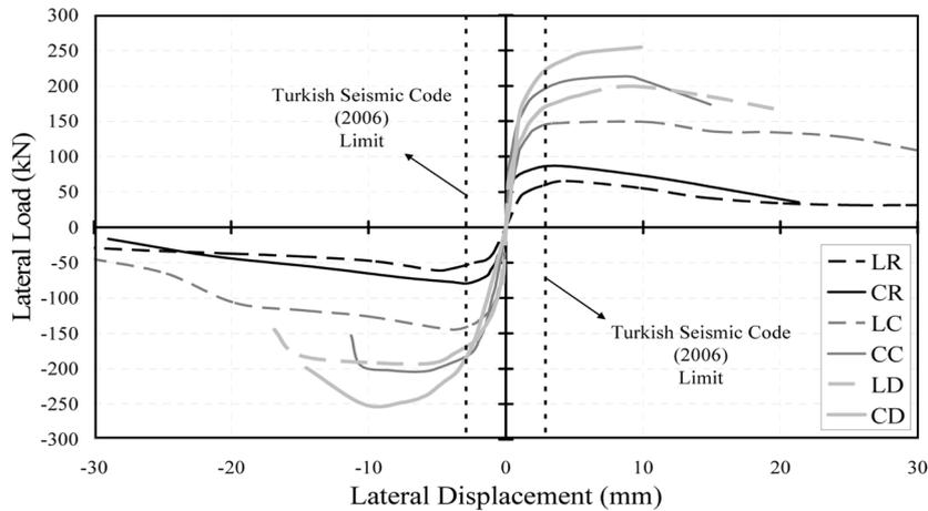
Fig. 12 Comparison for response envelopes of specimens having lap-splices with specimens having continuous column bars
