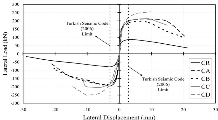
Fig. 11 Response envelopes of specimens having continuous column bars
