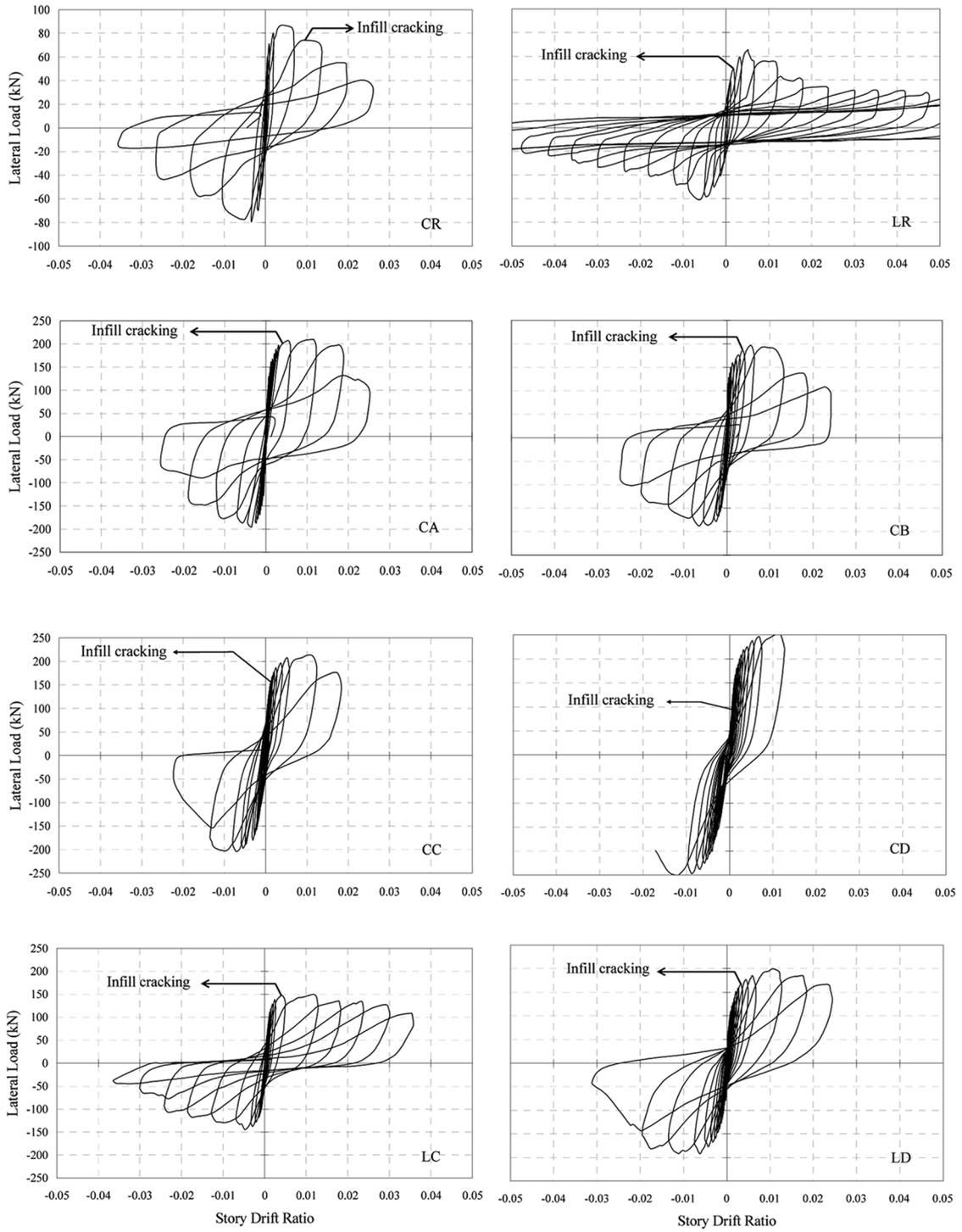
Fig. 9 Lateral load-story drift ratio curves
