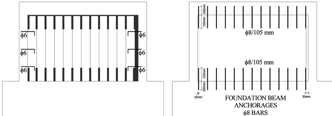
Fig. 6 Panel arrangement for Type D panels (Specimen CD and LD)
