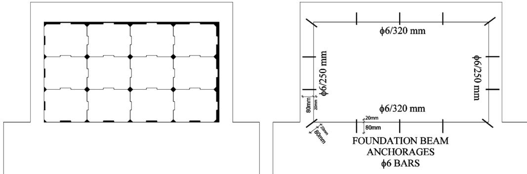
Fig. 3 Panel arrangement for Type A panels (Specimen CA)
