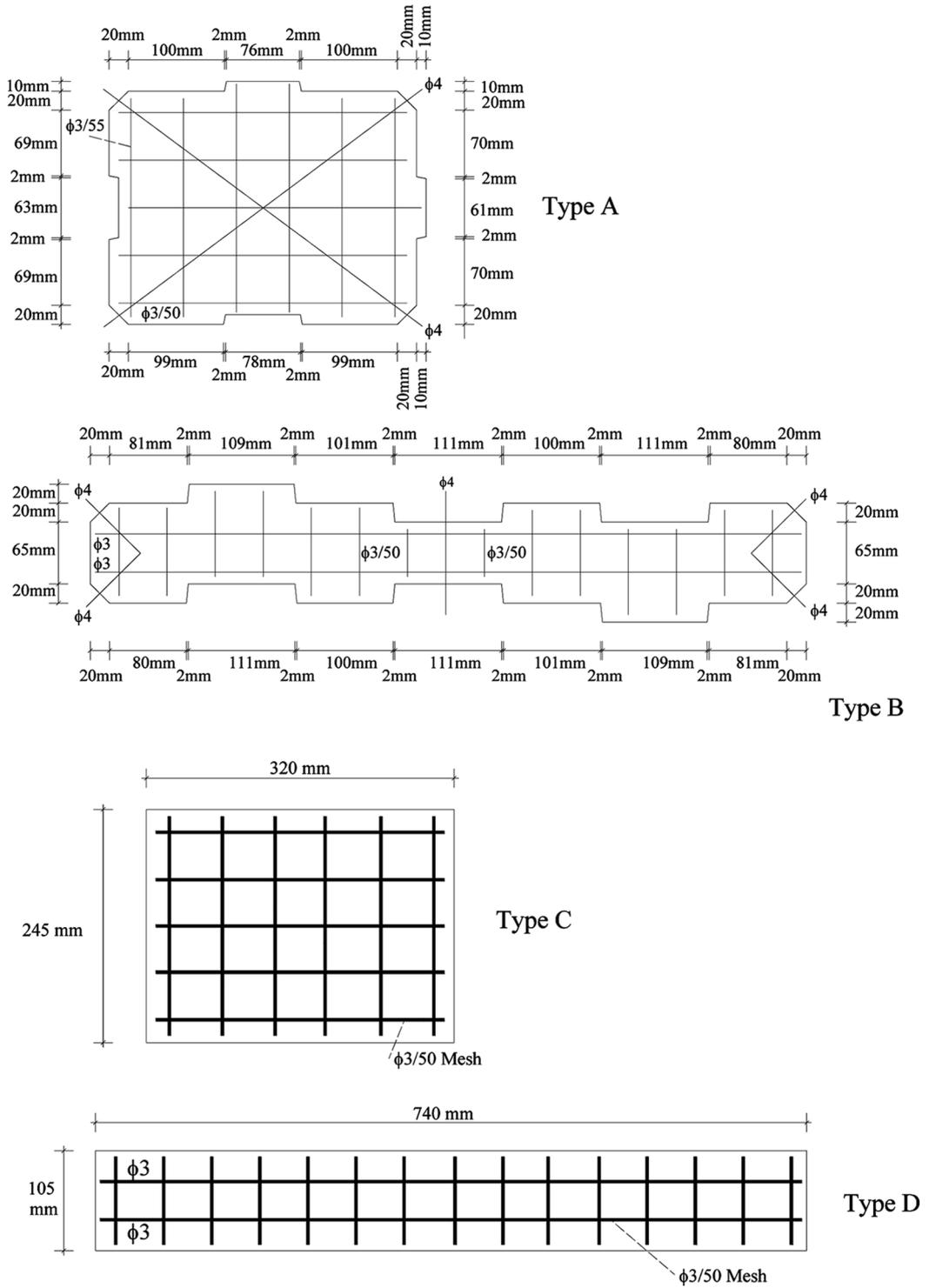
Fig. 2 Dimension and reinforcement of panel types
