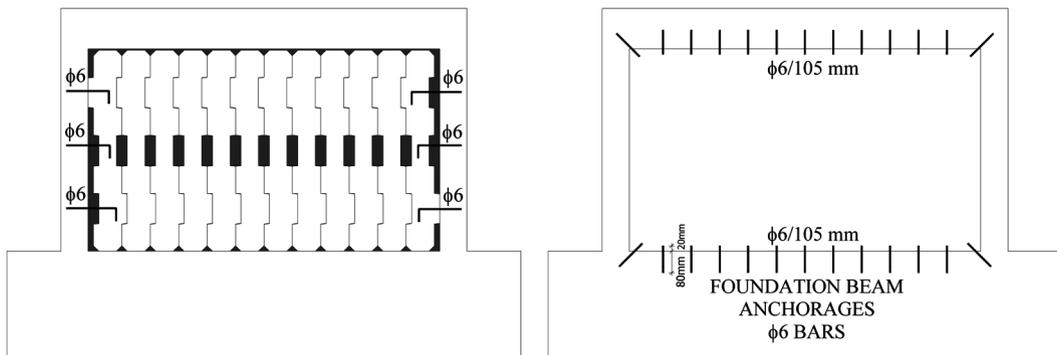
Fig. 4 Panel arrangement for Type B panels (Specimen CB)
