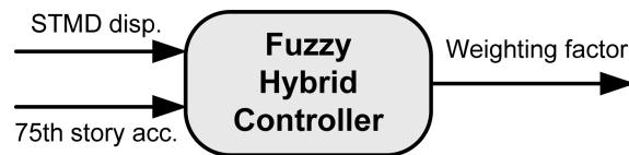
Fig. 7 Input and output relationships of fuzzy hybrid controller
