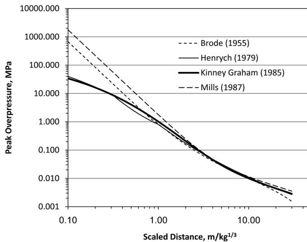
Fig. 2 Comparison of peak static overpressure prediction models
