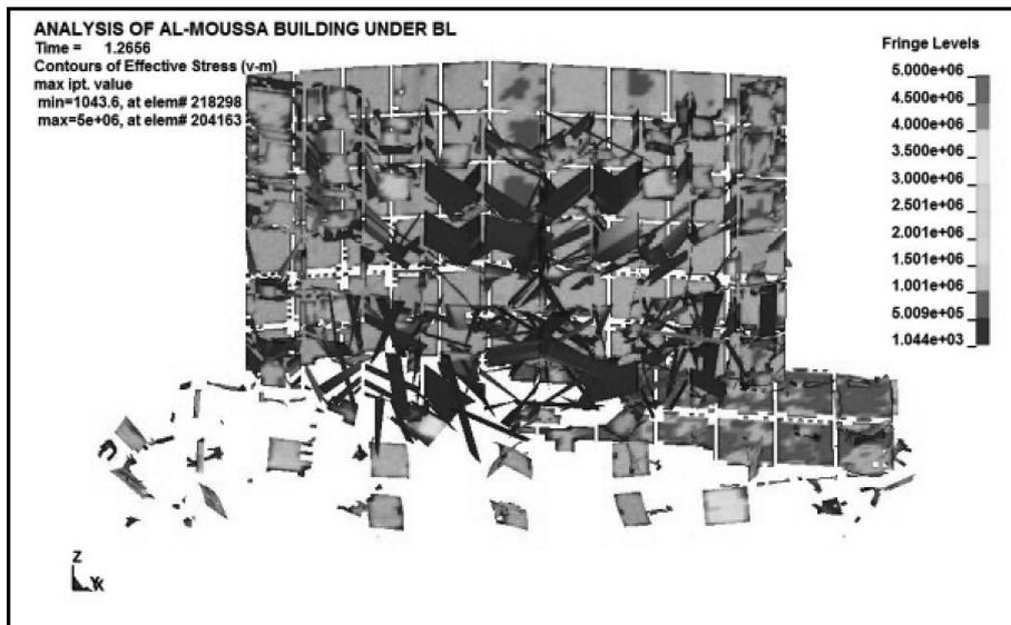
Fig. 10 Scenario 4: Damage caused to the glass and masonry facade of the building
