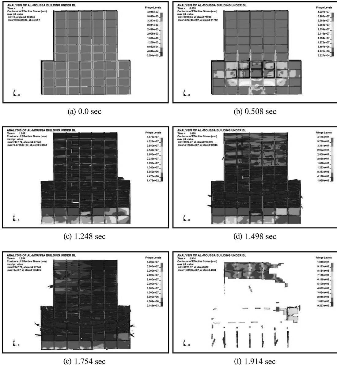
Fig. 6 Evolution of the structural damage produced by the explosion for Scenario 1
