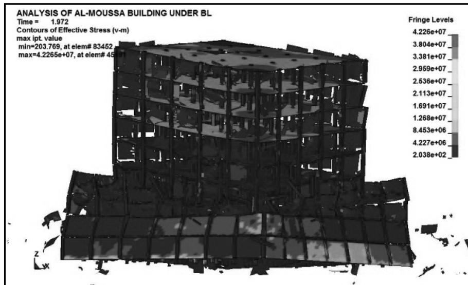
Fig. 8 Damage caused to the entire structure at 1.972 seconds Scenario 3
