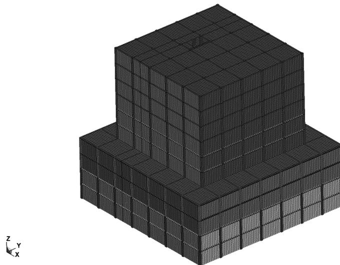
Fig. 3 Finite element geometry of the whole building
