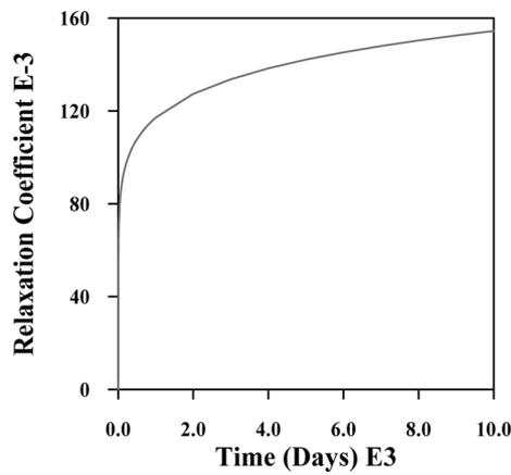
Fig. 10 Variation of time dependent material properties for prestressed steel
