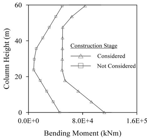
Fig. 15 Changing of bending moment along the height of the bridge column
