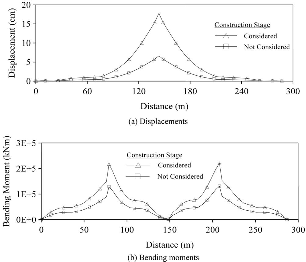
Fig. 12 Changing of maximum (a) displacements and (b) bending moments along the bridge deck
