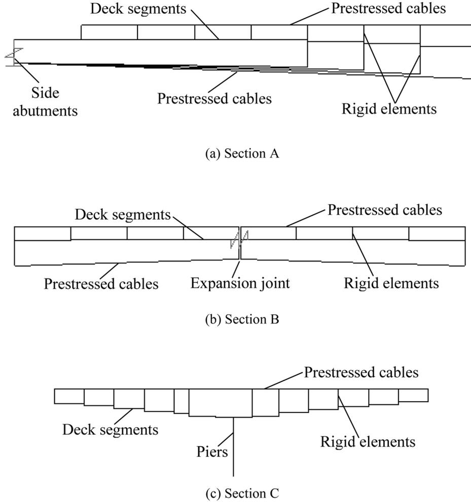
Fig. 7 Detailed presentation of section A, B and C
