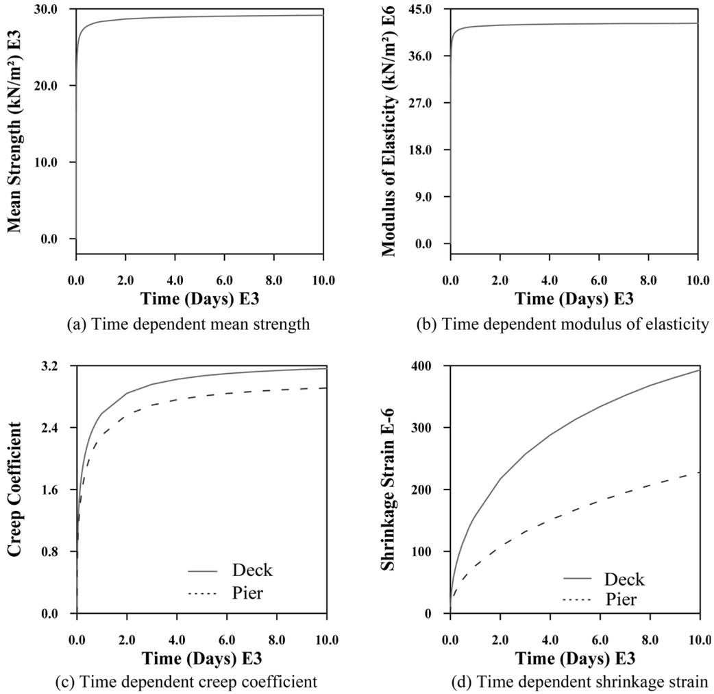
Fig. 9 Variation of time dependent material properties for concrete
