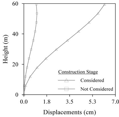
Fig. 13 Changing of displacements along the height of the bridge column
