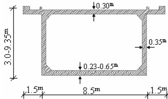
Fig. 3 Dimensions of box girder
