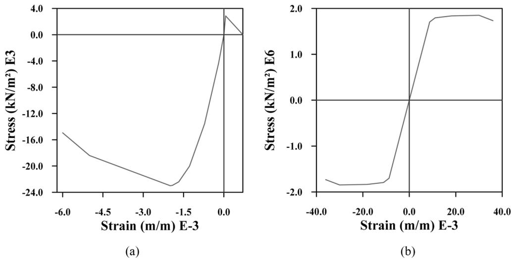
Fig. 8 Stress-strain diagrams used for (a) concrete and (b) prestressed steel
