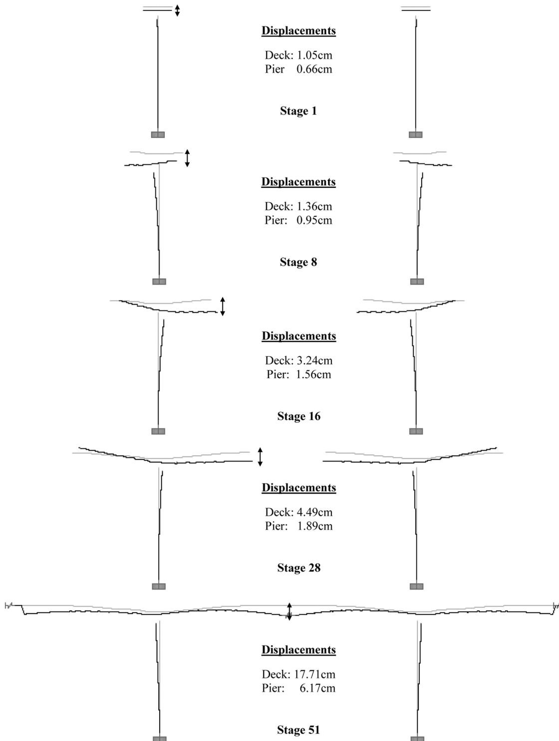
Fig. 11 Deformation of the highway bridge during some construction stages
