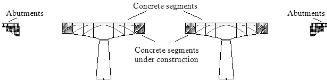
Fig. 5 The schematic view of balanced cantilever construction method
