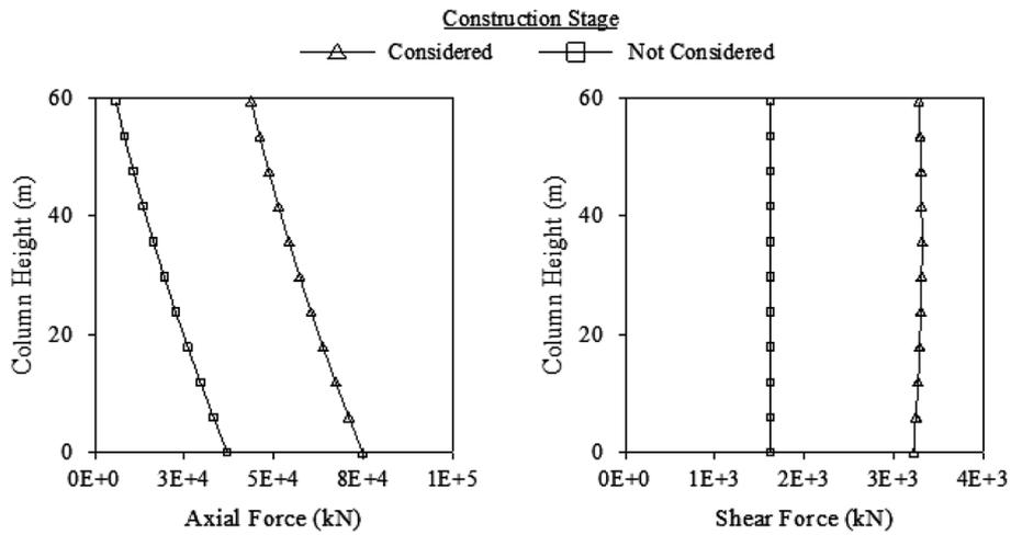
Fig. 14 Changing of internal forces along the height of the bridge column
