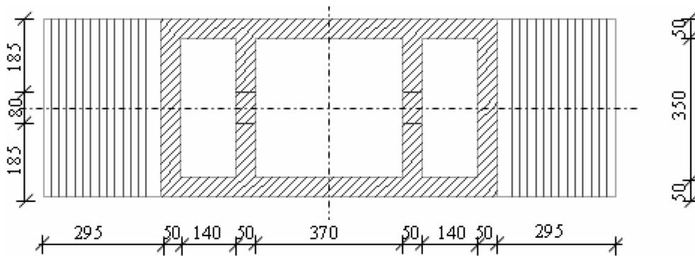
Fig. 4 Variable section of the main columns (dimensions as cm)
