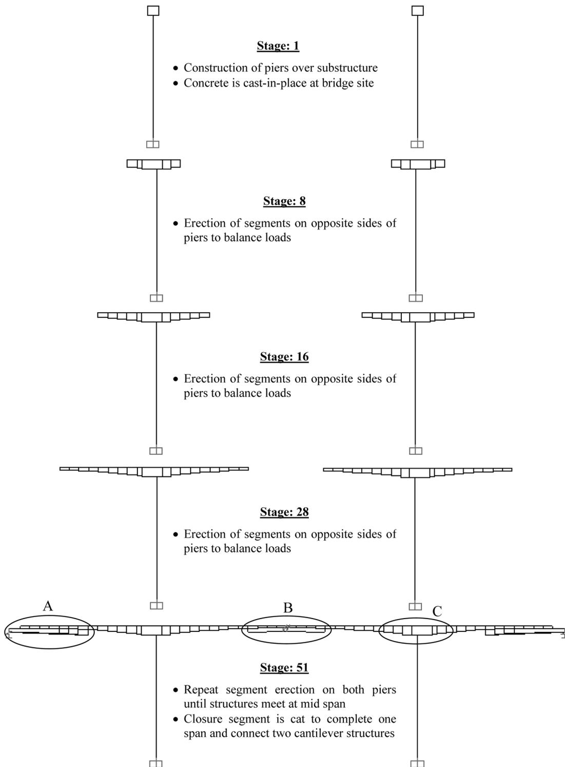
Fig. 6 Some construction stages of Kömürhan Highway Bridge
