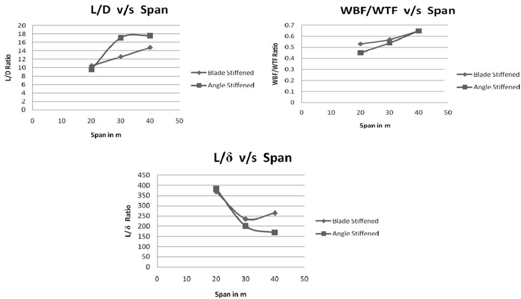
Fig. 5 Optimum value of dimension related parameters
