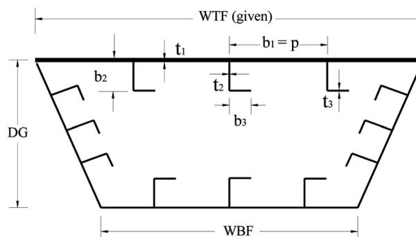
Fig. 1 Design variables of a box-girder section
