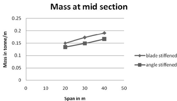
Fig. 4 Mid section mass v/s span
