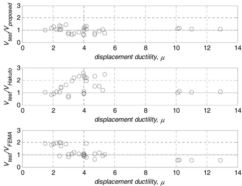
Fig. 2 Ratio of measured to calculated shear strength for the proposed, Hakuto and FEMA models versus displacement ductility
