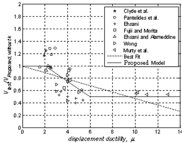
Fig. 1 Shear strength prediction as a function of displacement ductility, best fit linear line, and model representation
