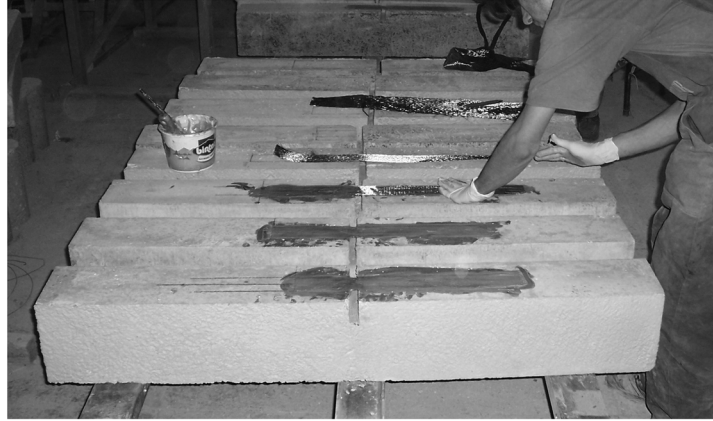
(a) A view of bonding of CFRP sheet
