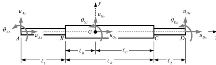
Fig. 2 A rigid beam segment BC connected with two elastic beam segments, AB and CD, at its two ends B and C, as shown in Fig. 1, can be replaced by a three-node elastic-and-rigid-combined beam element
