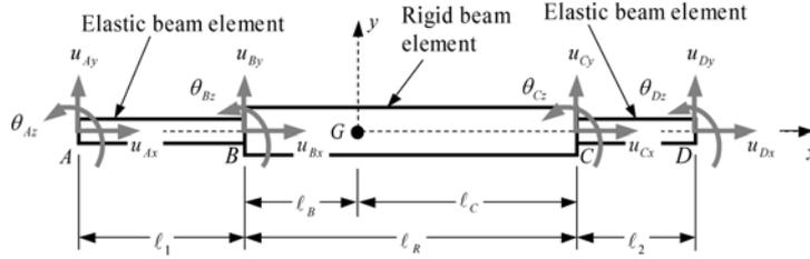
Fig. 1 A two-node rigid beam segment BC connected with two elastic beam segments, AB and CD, at its two ends B and C, respectively.
