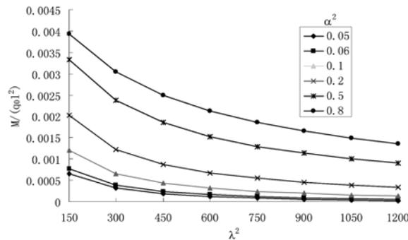
Fig. 8 Maximum bending moment under distributed load ( $q = 0.1q_0$ )
