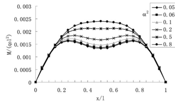
Fig. 4 Bending moment under the position of a concentrated load ( $\lambda^2 = 400$ )
