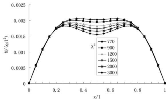
Fig. 2 Bending moment under the position of a concentrated load ( $\alpha^2 = 0.769$ )
