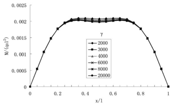
Fig. 6 Bending moment under the position of a concentrated load ( $\lambda^2 = 770, \alpha^2 = 0.77$ )
