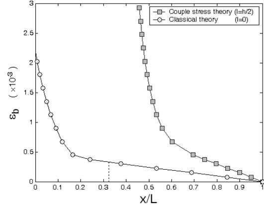
Fig. 3 The surface strain  $\varepsilon_b$  along the axial direction  $x$  for a cantilever beam. The beam thickness is  $h = 1 \mu\text{m}$ , the force applied at the free end is  $F = 0.6\text{N}$ , and the plastic work hardening exponent is  $m = 0.1$
