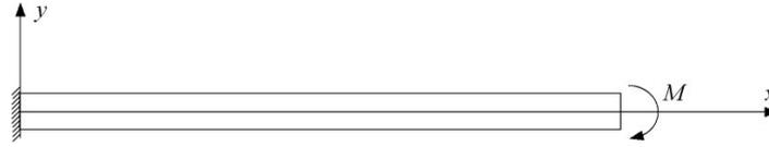
Fig. 1 Coordinate system  $(x, y)$  on a pure bending beam
