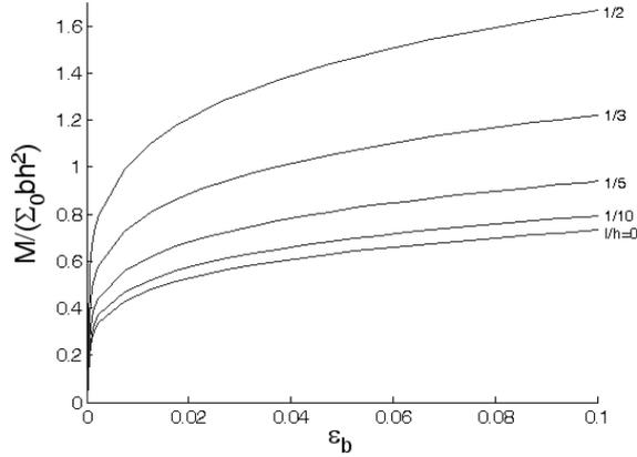
Fig. 2 The normalized moment  $M/\Sigma_0bh^2$  versus the surface strain  $\varepsilon_b = \kappa h/2$  with  $m = 0.2$
