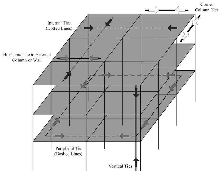
Fig. 2 Schematic of Tie Forces in a Frame Structure (Department of Defense, 2005)
