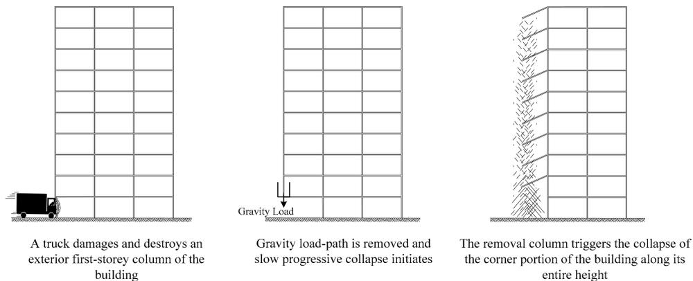
Fig. 1 Progressive collapse of a building caused by a truck accident
