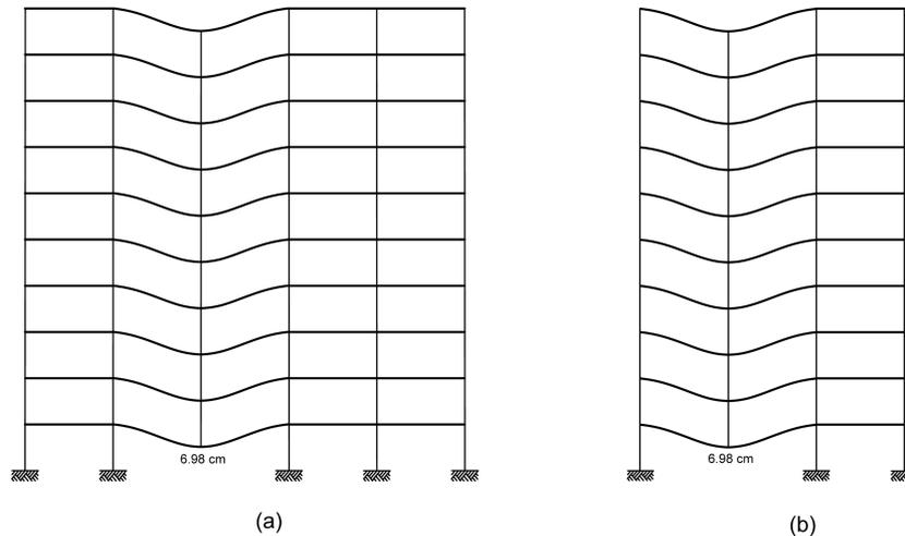
Fig. 5 Deflections obtained from progressive collapse analysis when first storey interior column is removed: (a) longitudinal frame and (b) transverse frame (Yagob 2007)
