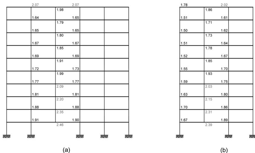
Fig. 4 Demand/Capacity ratios obtained from progressive collapse analysis, when first storey interior column is removed: (a) longitudinal frame and (b) transverse frame. (Values in light font indicate collapse according to GSA 2003 Guidelines) (Yagob 2007)
