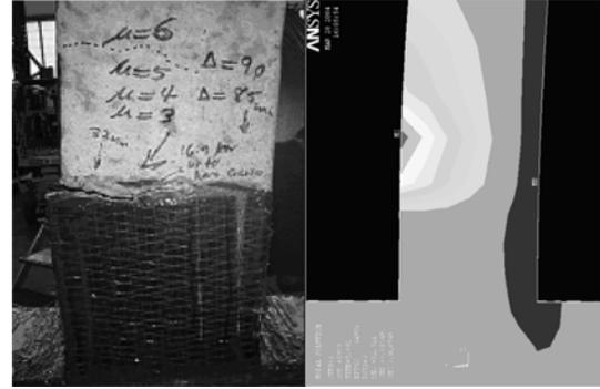
Fig. 17 Experimental versus numerical failure mechanism (RSM2)
