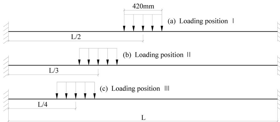
Fig. 4 Different positions of the localized blast loading
