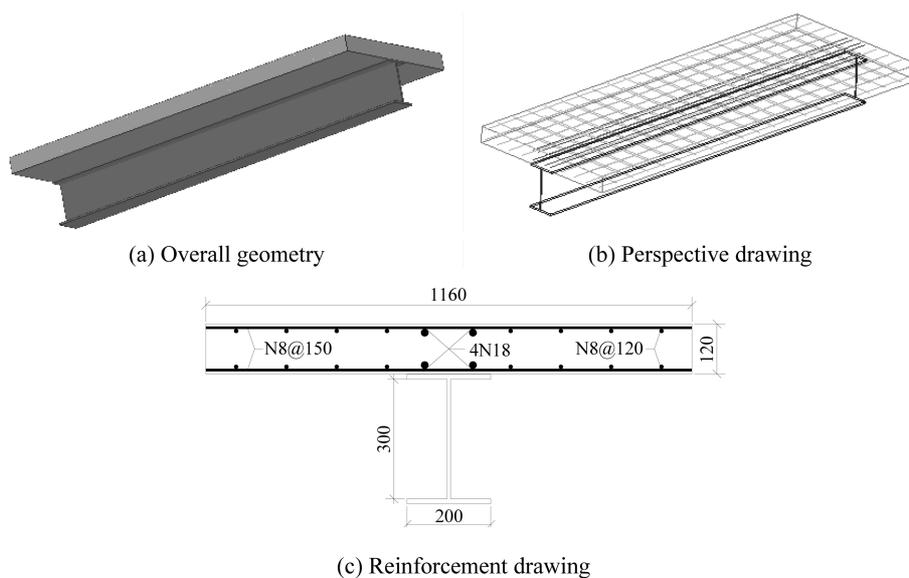
Fig. 3 Configuration of SCCB
