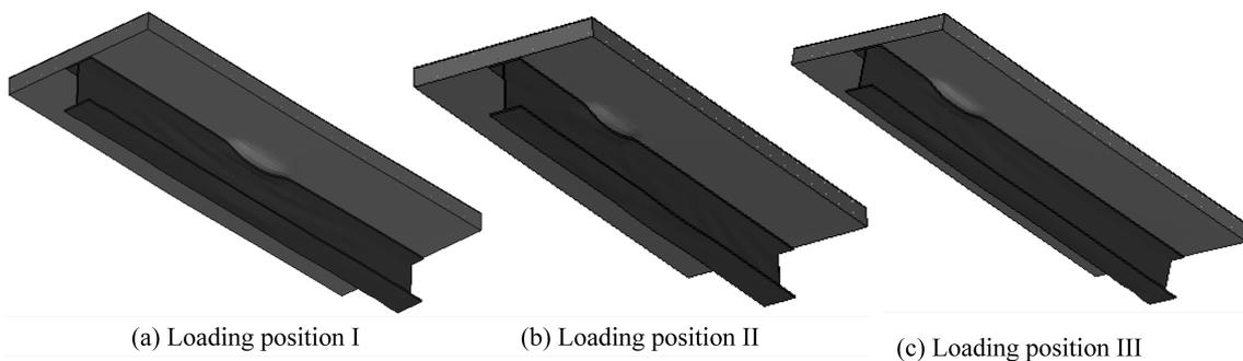
Fig. 5 Deformation profiles of SCCB under different loading positions
