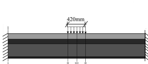
Fig. 2 SCCB under localized blast loading
