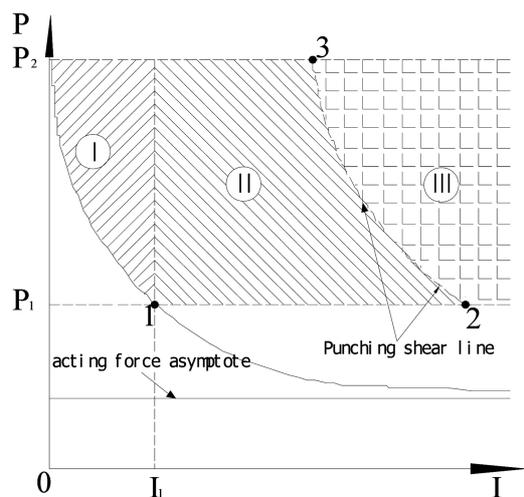
Fig. 8 Pressure-impulse diagram for failure modes of SCCB
