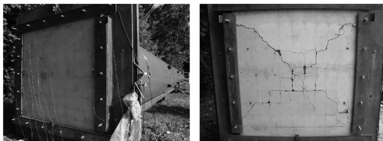
Fig. 2 (left) concrete slab in blast simulator, (right) extensive cracking after a blast load of 160 kPa peak pressure
