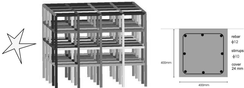
Fig. 9 (left) RC building under blast explosion; (right) cross section of columns and beams with reinforcement
