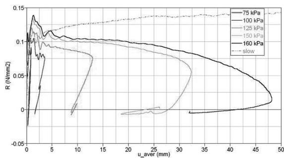
Fig. 4 Resistance-average displacement curves of reinforced concrete plate for blast pressures of 75-160 kPa (45 ms duration)
