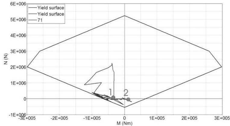
Fig. 14 M-N paths and yield surface of beam 71. The (1) and (2) points denote the pre-blast state and the end state respectively
