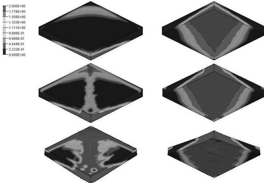
Fig. 6 Damage fields at  $t = 100$  ms, for three different blast pressures 75 kPa, 100 kPa and 150 kPa (45 ms duration); (left) pressure side and (right) back side
