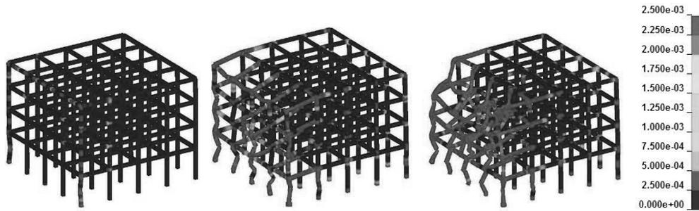
Fig. 16 Beams and columns: equivalent plastic strain plots for different blast charges, stand-off distance = 35 m: (above-left) 100 kg TNT; (above-right) 500 kg TNT; (below) 1000 kg TNT
