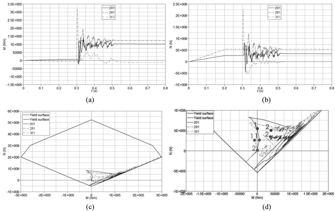
Fig. 13 Columns history variables. 1000 kg TNT, at 35 m standoff distance. (a) moment  $M$  history; (b) axial force  $N$  history; (c)  $M$ - $N$  trajectory and failure surface; (d) detailed plot, the (1) and (2) points denote the pre-blast state and the end state respectively
