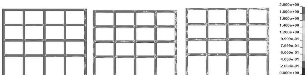
Fig. 19 Damage plots for different blast charges (stand-off distance = 35 m): (above-left) 100 kg TNT; (above-right) 500 kg TNT; (below) 1000 kg TNT
