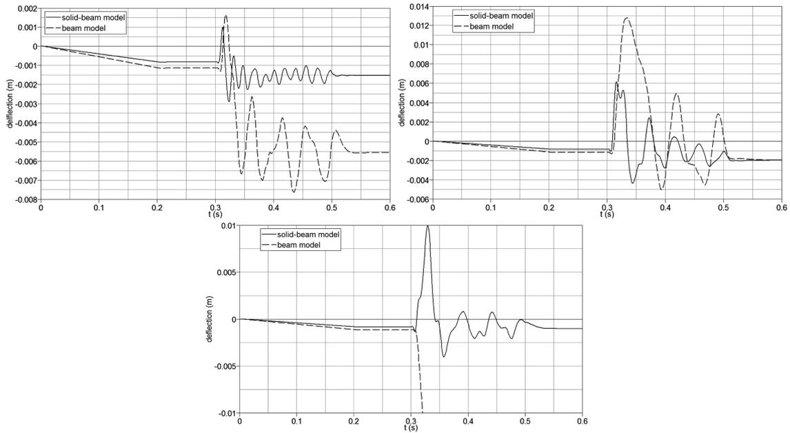
Fig. 20 Deflection history for the solid/beam (blue) and the beam smeared model (red). Stand-off distance = 35 m. (above-left) 100 kg TNT; (above-right) 500 kg TNT; (below) 1000 kg TNT
