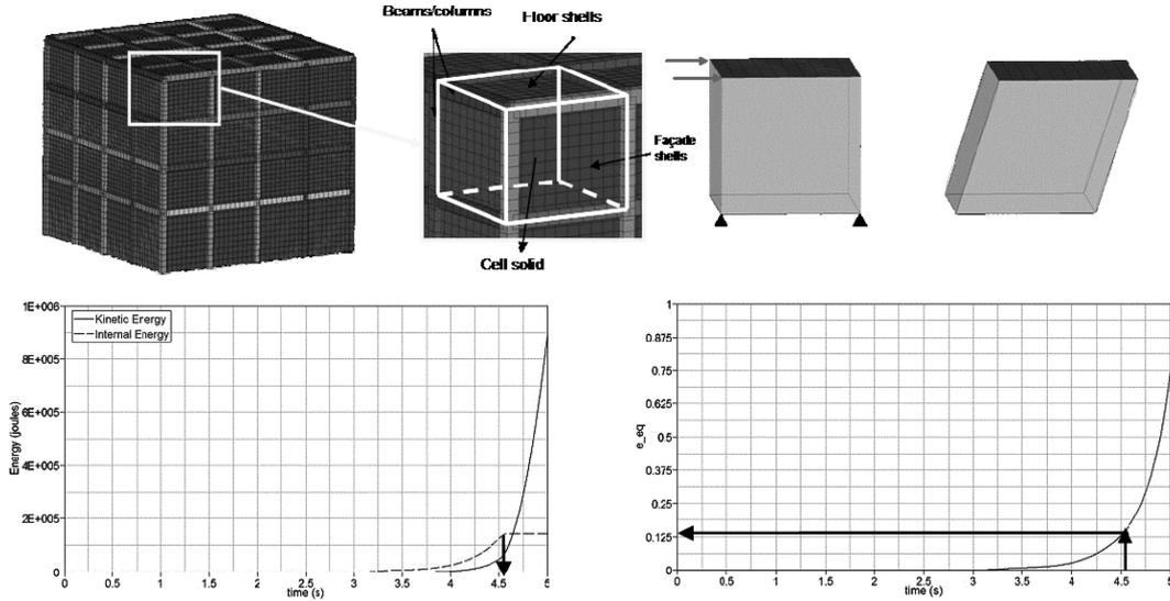
Fig. 21 Damage calibration procedure. (top left) a cell, consisting of structural and a volume ('gauge') element; (top-right) shear calibration test; (bottom-left) kinetic and internal energy history,  $U_{\max} = 1.2$  MJoules; (bottom-right) shear deformation history,  $\epsilon_{\max} = 0.13$
