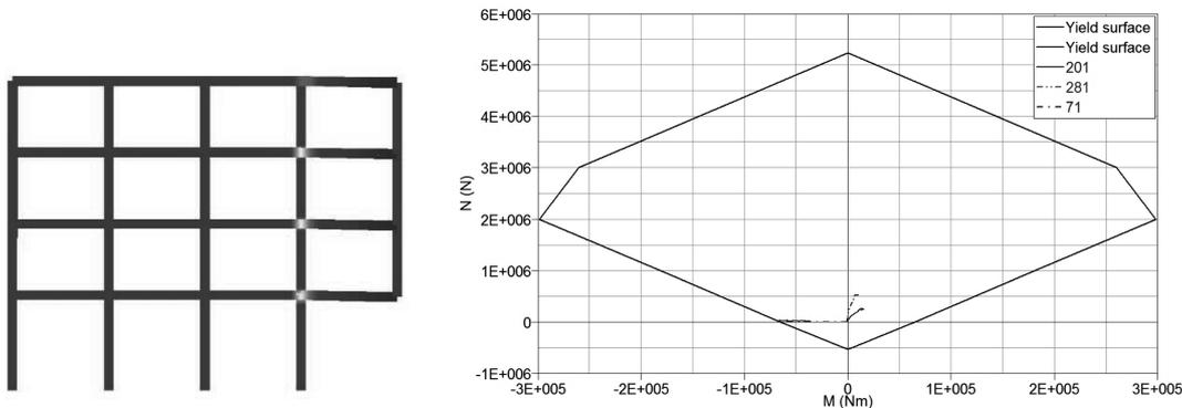
Fig. 15 Pseudo-static analysis for a 1000 kg TNT charge at 35 m standoff distance. (left) Equivalent plastic strain plot; (right) M-N trajectory and yield surface
