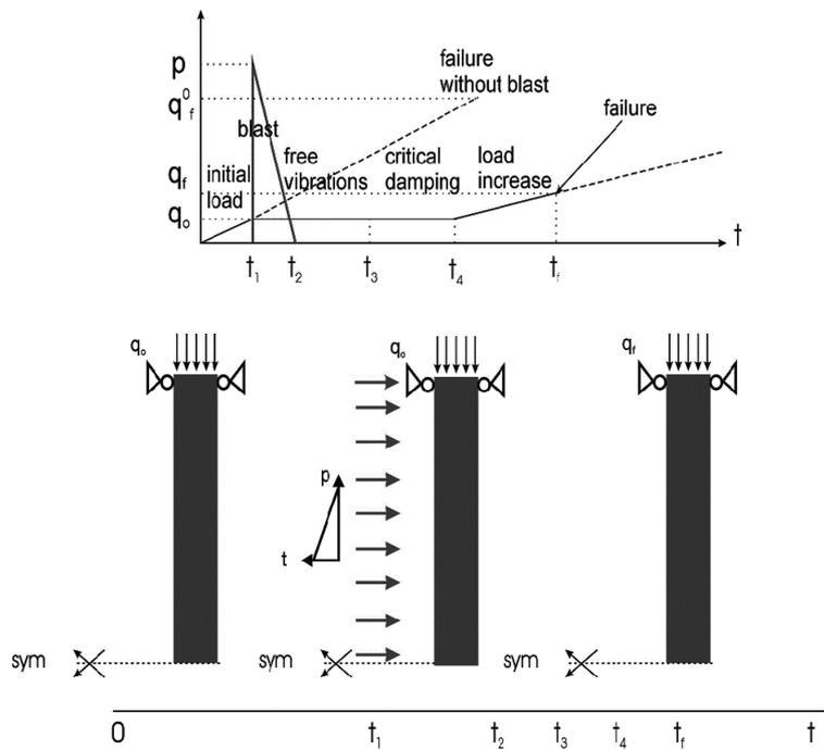
Fig. 8 Loading history to failure strength for a plate under static in-plane load and dynamic bending load
