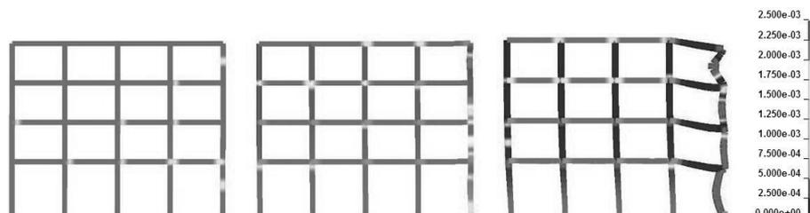
Fig. 11 Equivalent plastic strain plots for different blast charges (stand-off distance = 35 m): (above-left) 100 kg TNT; (above-right) 500 kg TNT; (below) 1000 kg TNT
