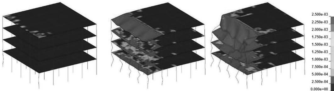
Fig. 17 Floors: equivalent plastic strain plots for different blast charges, stand-off distance=35 m: (above-left) 100 kg TNT; (above-right) 500 kg TNT; (below) 1000 kg TNT
