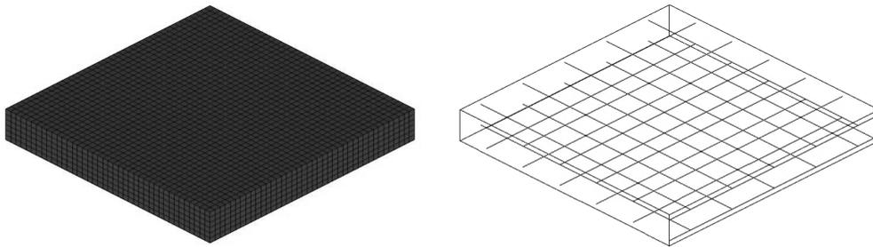
Fig. 3 (left) half mesh with double solid elements (concrete ) and (right) rebars
