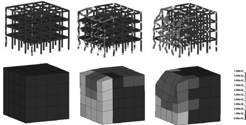
Fig. 22 Illustration of the relation between the structural damage and the damage indicator for the three different blast charges: (left) 100 kg, (middle) 500 kg, (right) 1000 kg of TNT
