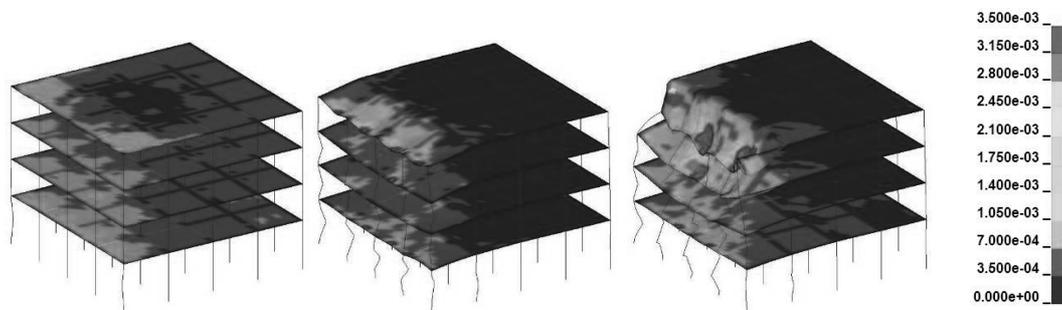
Fig. 18 Floors: uniaxial concrete strain plots for different blast charges, stand-off distance=35 m: (above-left) 100 kg TNT; (above-right) 500 kg TNT; (below) 1000 kg TNT
