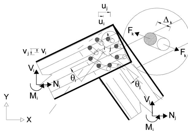
Fig. 3 Connection element
