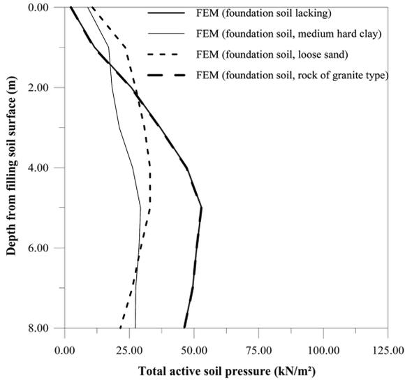
Fig. 15 Total active soil pressure distributions of the retaining wall calculated according to the finite element method for different foundation soil type
