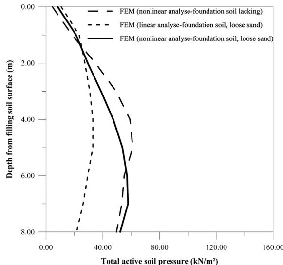
Fig. 17 Total active soil pressure distributions of the retaining wall calculated according to the finite element method for the cases considering or not considering foundation interaction
