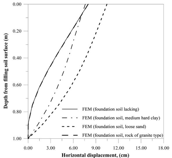
Fig. 16 Horizontal displacements of the retaining wall calculated according to the finite element method for different foundation soil type
