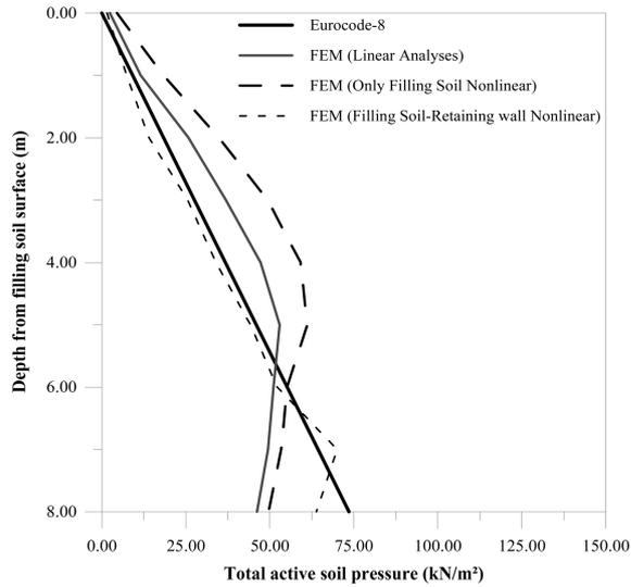
Fig. 12 Total active soil pressure distributions of the retaining wall calculated according to the method suggested in Eurocode-8 and the finite element method for linear and nonlinear analyses
