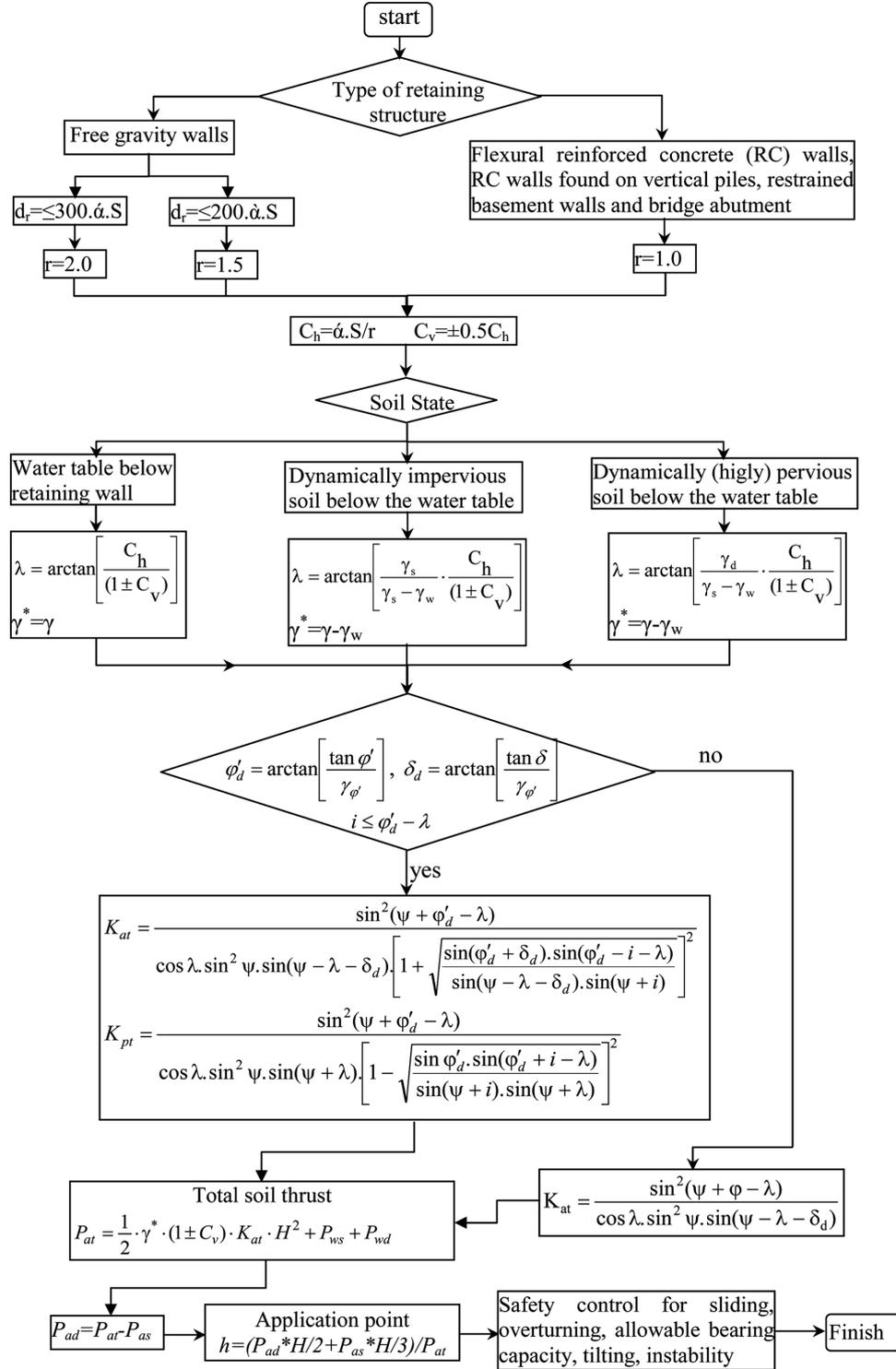
Fig. 3 The flow-chart diagram of designing of retaining walls according to Eurocode-8
