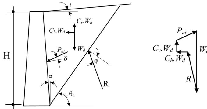
Fig. 2 Forces acting on active wedge according to Mononobe-Okabe Method
