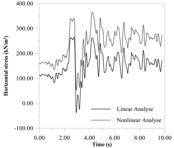
Fig. 13 Time history of normal stress at 638 node point in model 1 of the retaining wall for linear and nonlinear analyses
