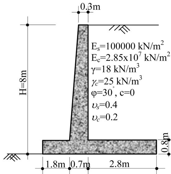
Fig. 7 Example for retaining wall and soil parameters
