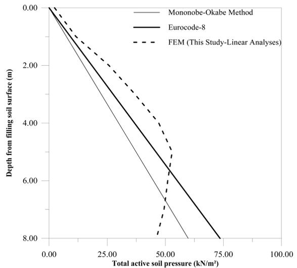
Fig. 10 Total active soil pressure distributions acting on the retaining wall due to the earthquake according to different methods
