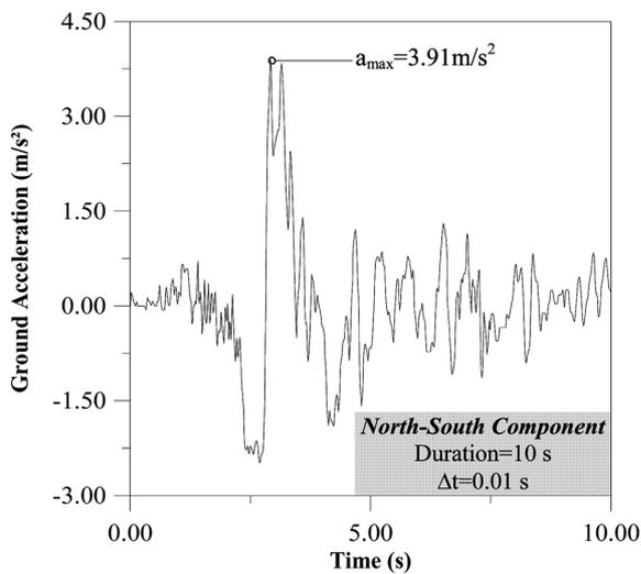
Fig. 9 Ground acceleration of North-South component of March 13, 1992 Erzincan earthquake
