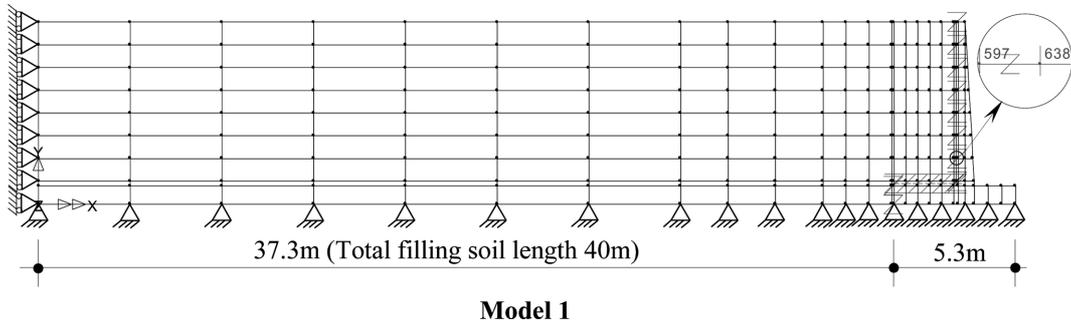
Fig. 8 Finite element mesh used for two dimensional analyses to filling soil-retaining wall interaction
