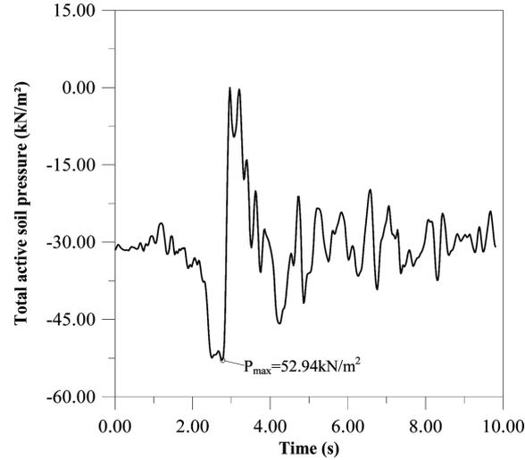
Fig. 11 Time history of total active soil pressure of the retaining wall at 638 node point in model 1
