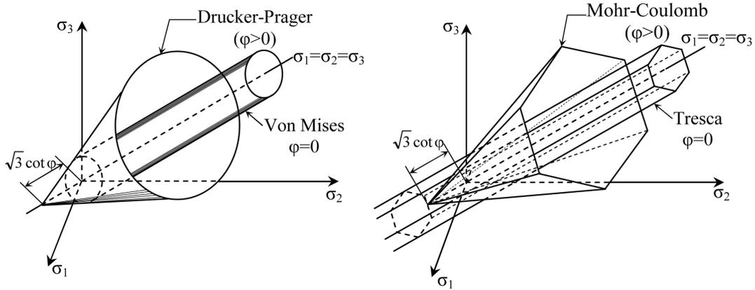
Fig. 5 Schematic failure surfaces at the principal stress space for different failure criteria
