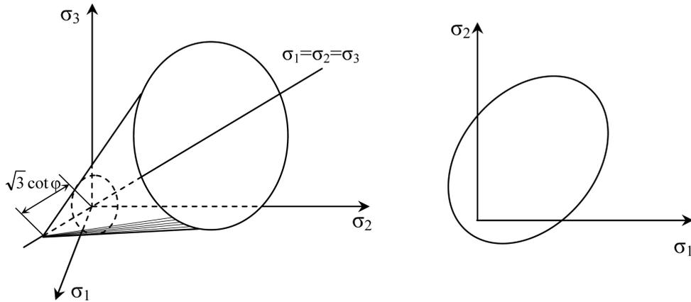
Fig. 6 Drucker-Prager schematic failure surfaces at two dimensional principal stress planes and at three dimensional principal stress spaces
