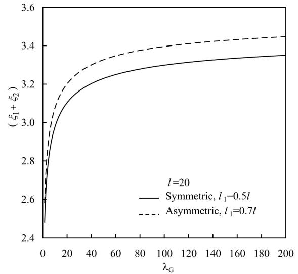
Fig. 11 Variation of total contact length with the shear foundation parameter  $\lambda_G$  for  $F = 0.1$  and  $l = 20$ , for the symmetric and asymmetric case in the pinned-pinned beam
