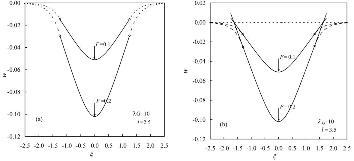
Fig. 3 Deflection curves for the free-free beam under two different symmetric loads with  $\lambda_G = 10$ . (a)  $l = 2.5$ , (b)  $l = 3.5$
