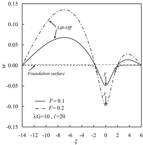
Fig. 10 Deflection curves for the pinned-pinned beam under two different loads with  $l = 20$  and  $\lambda_G = 10$
