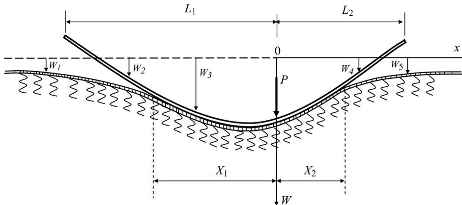
Fig. 1 Finite beam on a tensionless Pasternak foundation subjected to an eccentric load
