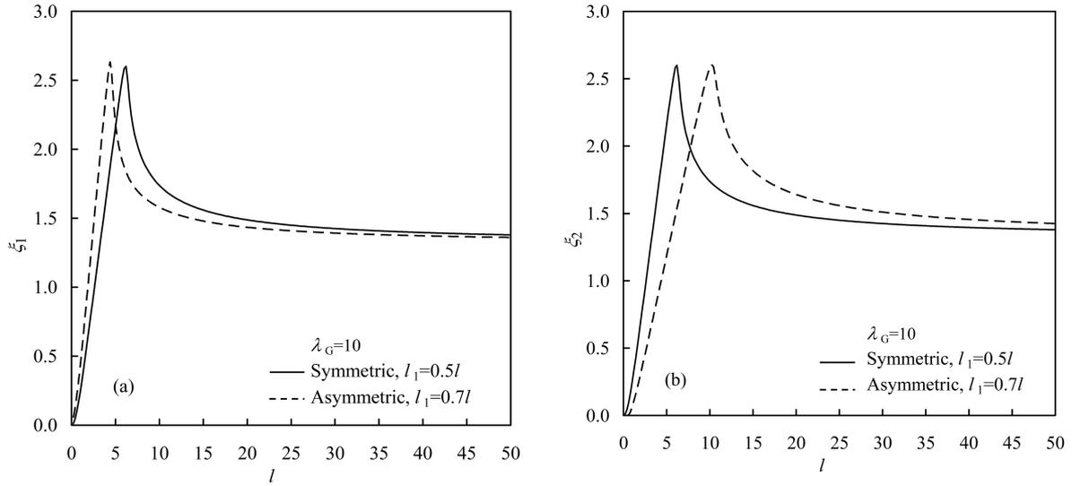
Fig. 9 Contact lengths versus beam length for  $F = 0.1$  and  $\lambda_G = 10$ , for the symmetric and asymmetric case in the pinned-pinned beam. (a) Left side ( $\xi_1$ ), (b) Right side ( $\xi_2$ )
