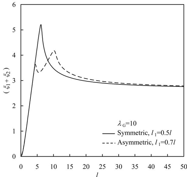
Fig. 8 Variation of total contact length ( $\xi_1 + \xi_2$ ) with beam length  $l$  for  $F = 0.1$  and  $\lambda_G = 10$ , for the symmetric and asymmetric case in the pinned-pinned beam
