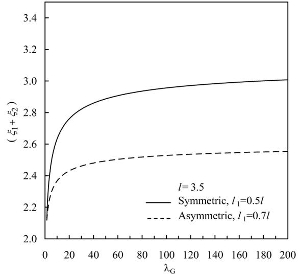
Fig. 6 Variation of total contact length ( $\xi_1 + \xi_2$ ) with the shear foundation parameter  $\lambda_G$  for  $F = 0.1$  and  $l = 3.5$ , for the symmetric and asymmetric case in the free-free beam
