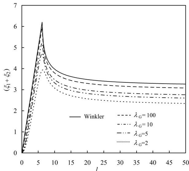
Fig. 7 Variation of total contact length ( $\xi_1 + \xi_2$ ) with beam length  $l$  for  $F = 0.1$  and some values of  $\lambda_G$ , for the symmetric loading case in the pinned-pinned beam
