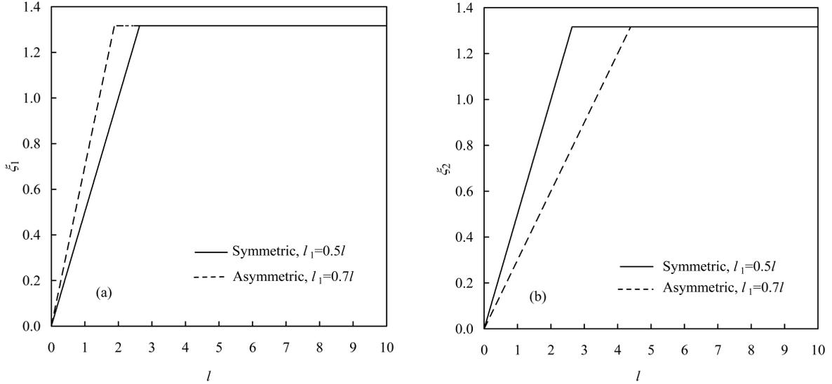
Fig. 4 Contact lengths versus beam length for  $F = 0.1$  and  $\lambda_G = 10$ , for the symmetric and asymmetric case in the free-free beam. (a) Left side ( $\xi_1$ ); (b) Right side ( $\xi_2$ )
