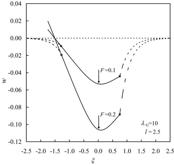
Fig. 5 Deflection curves for the free-free beam under two different asymmetric loads with  $l = 2.5$  and  $\lambda_G = 10$
