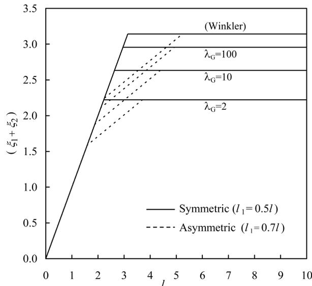
Fig. 2 Variation of total contact length ( $\xi_1 + \xi_2$ ) with beam length  $l$  for  $F = 0.1$  and some values of  $\lambda_G$ , for the symmetric and asymmetric loading in the free-free beam case
