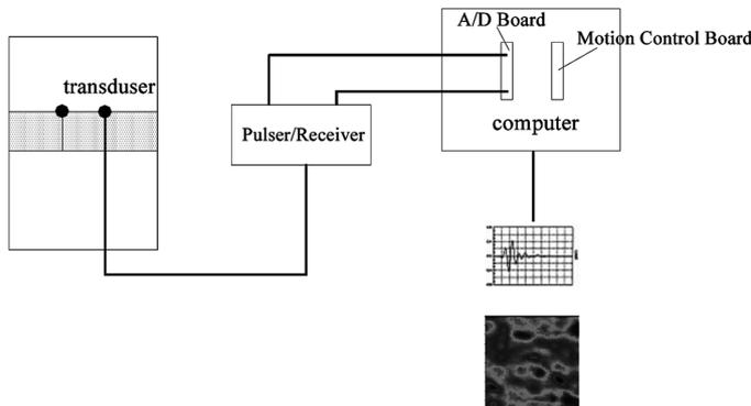
Fig. 1 Scan system transmission and control configuration
