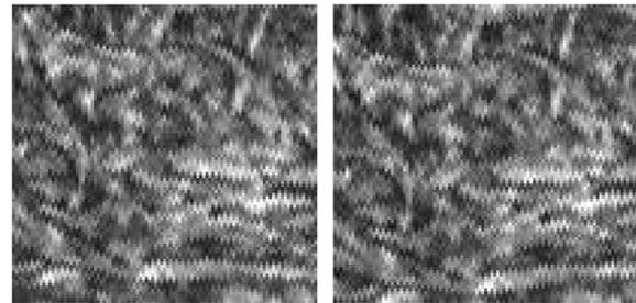
Fig. 2 Typical “before” and “after” C-scan images used to find displacement, rotation and strain
