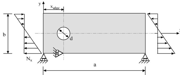
Fig. 1 Geometry of a plate with a circular hole
