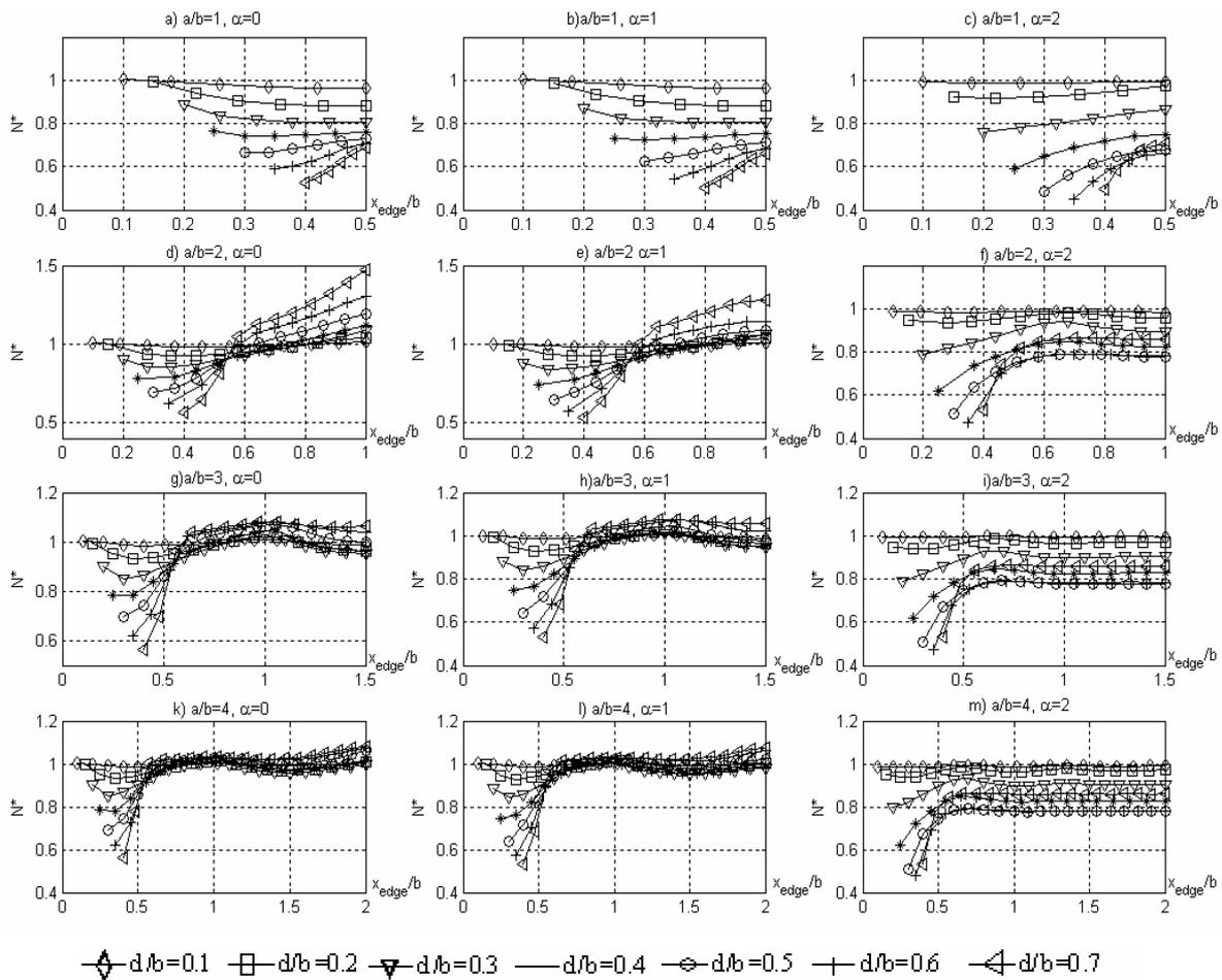
Fig. 2 Buckling load ratios  $N^*(=N/N_{cr})$  for square plates with circular holes moving along the major axis and subjected to different loading cases
