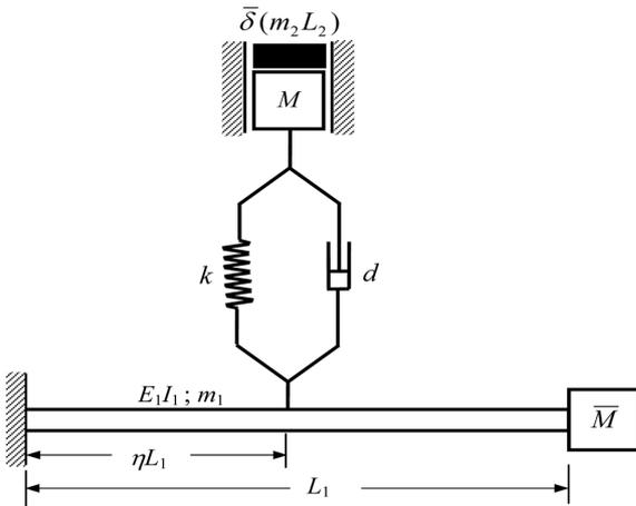
Fig. 3 Simplified representation of the vibrational system in Fig. 1
