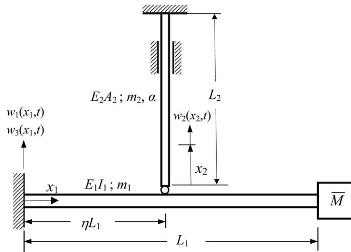
Fig. 2 Vibrational system in Fig. 1 for the limit  $M \rightarrow \infty$  (i.e.,  $\alpha_M \rightarrow \infty$ )
