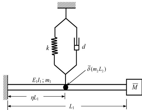
Fig. 4 Simplified representation of the vibrational system in Fig. 2
