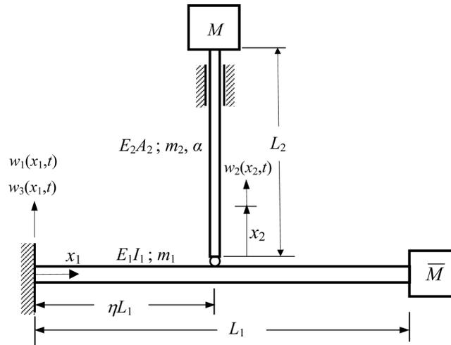
Fig. 1 Vibrational system under study: A cantilevered beam with a tip mass and in-span an axially vibrating visco-elastic rod with a tip mass
