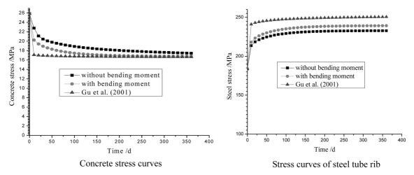
Fig. 4 Stress curves at mddle span of arch rib
