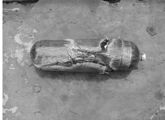
Fig. 7 Burst test of FRP vessel under 114 MPa hydrostatic pressure
