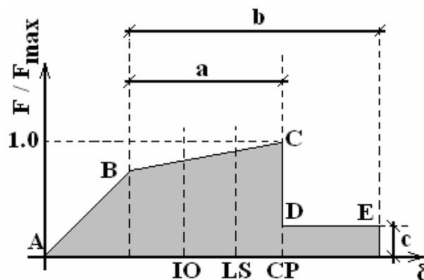
Fig. 9 Idealized force versus deformation curve for the deformation-controlled components from FEMA-356
