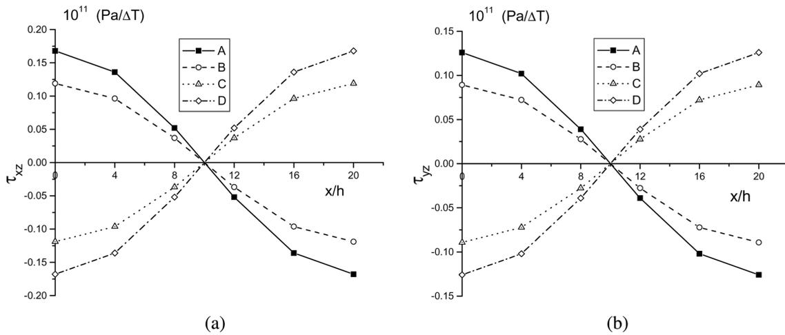
Fig. 8 (a,b) The response histories and distribution of interlaminar stress in laminated plates with the stacking sequence  $[45^\circ/-45^\circ]_s$ , under vibration mode of  $\omega_{21} = 412$  rad/s. The curves A, B, C and D represent, respectively, the interlaminar stresses at times  $t = 0.5 \omega_{21} \pi$ ,  $t = 0.75 \omega_{21} \pi$ ,  $t = 1.25 \omega_{21} \pi$  and  $t = 1.5 \omega_{21} \pi$
