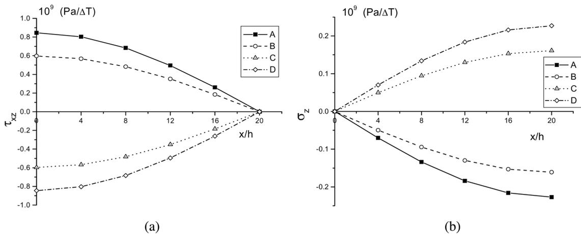
Fig. 5 (a,b) The response histories and distribution of interlaminar stress in laminated plates with the stacking sequence  $[90^\circ/0^\circ]_s$ , under vibration mode of  $\omega_{11} = 138$  rad/s. The curves A, B, C and D represent, respectively, the interlaminar stresses at times  $t = 0.5 \omega_{11}\pi$ ,  $t = 0.75 \omega_{11}\pi$ ,  $t = 1.25 \omega_{11}\pi$  and  $t = 1.5 \omega_{11}\pi$
