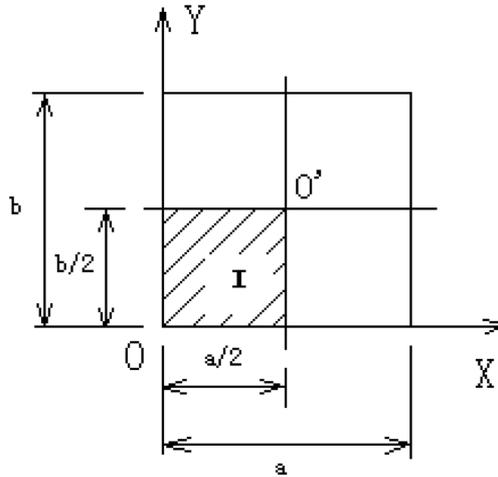
Fig. 2 The plane structure of the laminated plates with simply supported edges. I represents 1/4 symmetry region of the laminated plates
