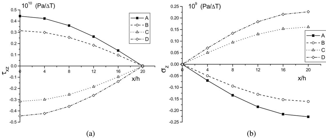
Fig. 3 (a,b) The response histories and distribution of interlaminar stress in laminated plates with the stacking sequence  $[0^9/90^9]_s$ , under vibration mode of  $\omega_{11} = 138$  rad/s. The curves A, B, C and D represent, respectively, the interlaminar stresses at times  $t = 0.5 \omega_{11} \pi$ ,  $t = 0.75 \omega_{11} \pi$ ,  $t = 1.25 \omega_{11} \pi$  and  $t = 1.5 \omega_{11} \pi$
