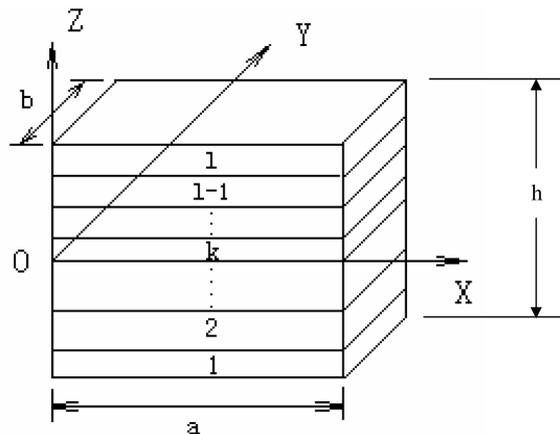
Fig. 1 The structure of rectangular orthotropic laminated plates with simply supported edges
