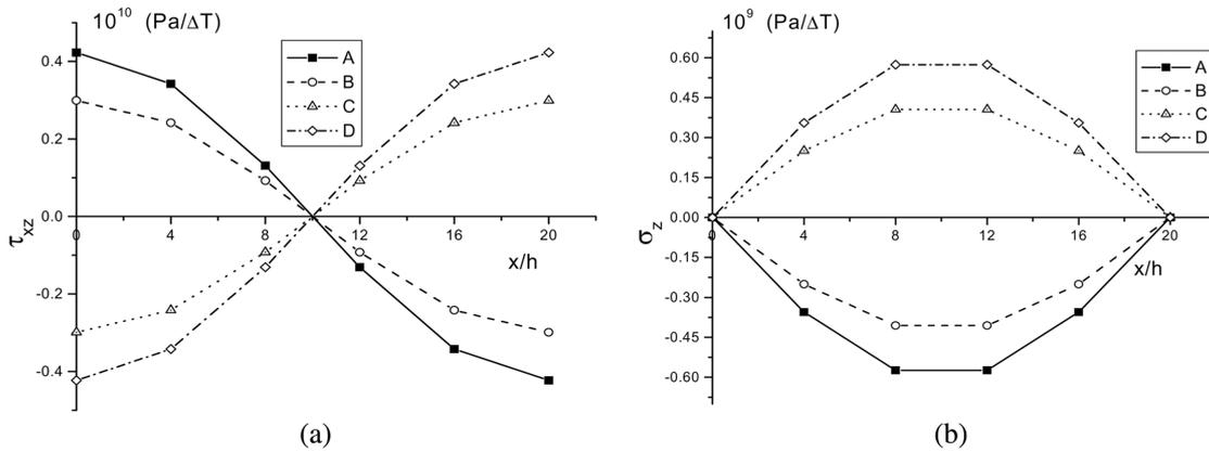
Fig. 6 (a,b) The response histories and distribution of interlaminar stress in laminated plates with the stacking sequence  $[90^\circ/0^\circ]_s$ , under vibration mode of  $\omega_{21} = 274$  rad/s. The curves A, B, C and D represent, respectively, the interlaminar stresses at times  $t = 0.5 \omega_{21} \pi$ ,  $t = 0.75 \omega_{21} \pi$ ,  $t = 1.25 \omega_{21} \pi$  and  $t = 1.5 \omega_{21} \pi$
