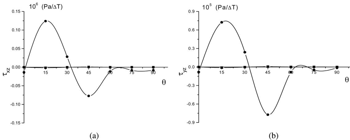
Fig. 9 (a,b) The distributions of interlaminar stresses at  $x = 20 h$ ,  $y = 20 h$ , and  $z = h$ , with the change of the stacking angle  $[\pm\theta]$ , under the vibration mode of  $\omega_{11}$
