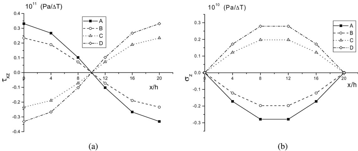
Fig. 4 (a,b) The response histories and distribution of interlaminar stress in laminated plates with the stacking sequence  $[0^\circ/90^\circ]_s$ , under vibration mode of  $\omega_{21} = 469$  rad/s. The curves A, B, C and D represent, respectively, the interlaminar stresses at times  $t = 0.5 \omega_{21}\pi$ ,  $t = 0.75 \omega_{21}\pi$ ,  $t = 1.25 \omega_{21}\pi$  and  $t = 1.5 \omega_{21}\pi$
