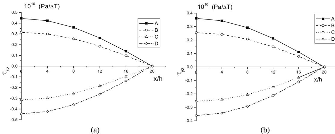
Fig. 7 (a,b) The response histories and distribution of interlaminar stress in laminated plates with the stacking sequence  $[45^\circ/-45^\circ]_s$ , under vibration mode of  $\omega_{11} = 178$  rad/s. The curves A, B, C and D represent, respectively, the interlaminar stresses at times  $t = 0.5 \omega_{11} \pi$ ,  $t = 0.75 \omega_{11} \pi$ ,  $t = 1.25 \omega_{11} \pi$  and  $t = 1.5 \omega_{11} \pi$
