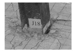
Fig. 12 Crush of concrete around column
