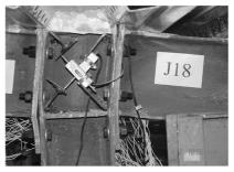
(d) Separation between end plate and column flange of J18
