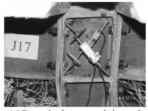
(a) Separation between end plate and column flange of J17
