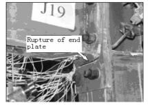
(f) Welding failure of J19
