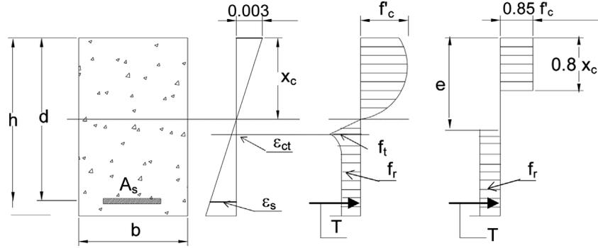
Fig. 4 Equilibrium of the transverse cross-section
