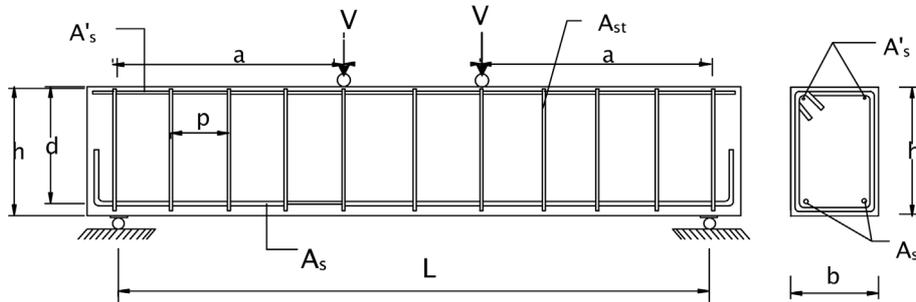
Fig. 1 Static scheme of the beam
