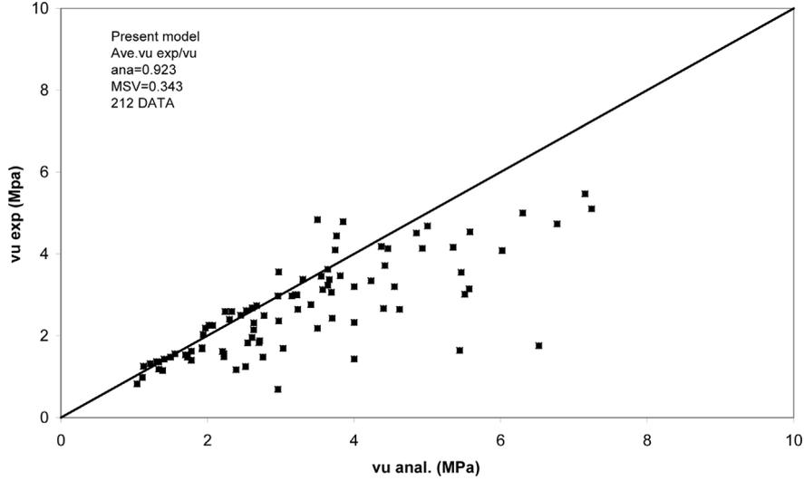
Fig. 7 Comparison between analytical and experimental results for fibrous concrete beam
