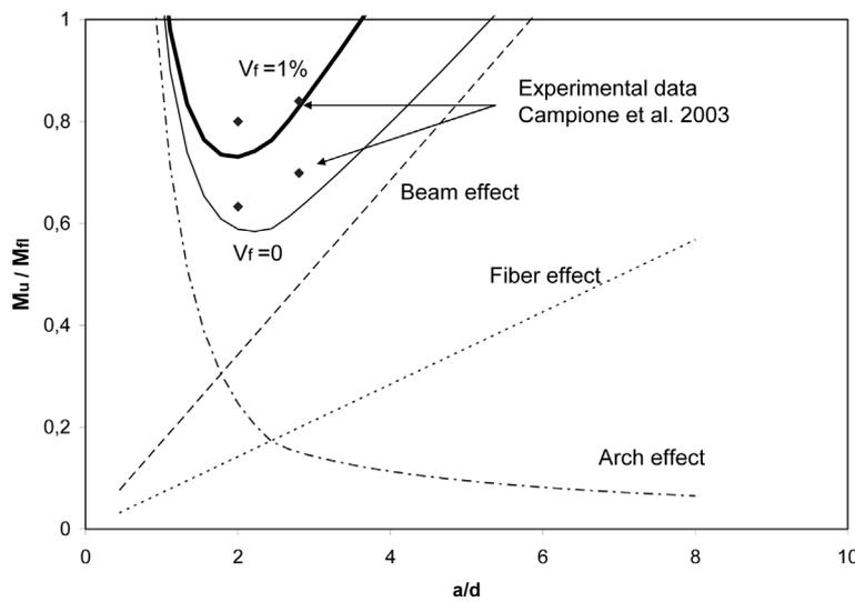
Fig. 8 Relative flexural capacity for fibrous concrete beam
