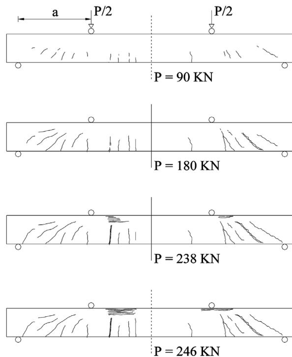
Fig. 15 Evolution of the cracks up to failure of a beam with  $V_f = 2\%$ ,  $p = 200 \text{ mm}$  and  $a/d = 2.8$  (Campione *et al.* 2003)
