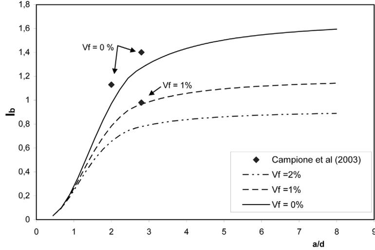
Fig. 10 Variation in the  $I_b$  with  $a/d$  for plain and fibrous concrete beams
