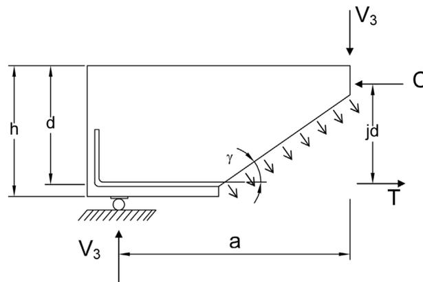
Fig. 6 Strength mechanism due to fiber across the principal crack
