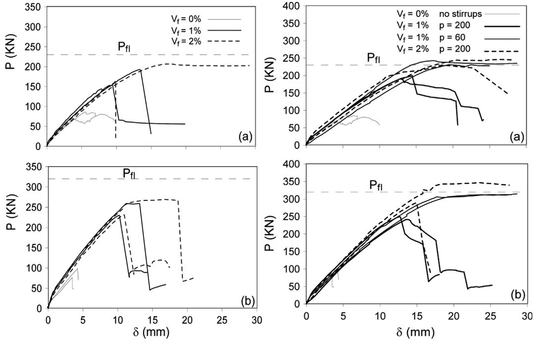
Fig. 13 Load-deflection curves for fibrous concrete beams with and without stirrups: (a)  $a/d = 2.8$ , (b)  $a/d = 2$ , (Campione *et al.* 2003)
