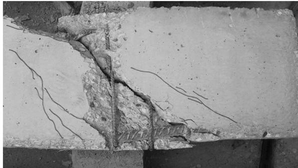
Fig. 14 Shear failure of a beam with stirrups at pitch 60 mm and for  $a/d = 2.0$
