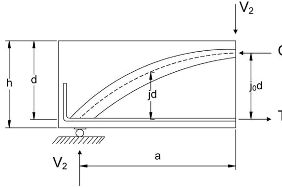
Fig. 5 Strength mechanism due to arch action
