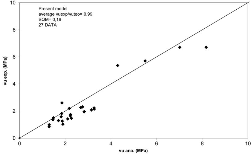
Fig. 11 Comparison between analytical and experimental results for fibrous concrete beams with stirrups
