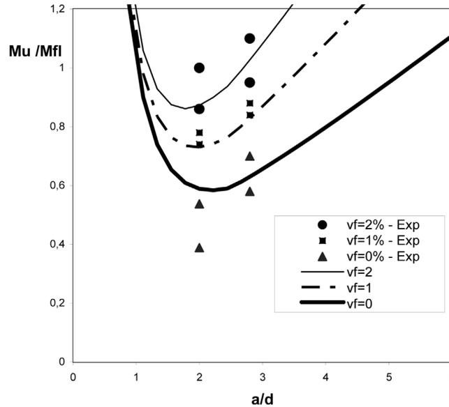
Fig. 16 Flexural relative capacity with the variation of  $a/d$  and  $p = 200$  mm (Campione *et al.* 2003)
