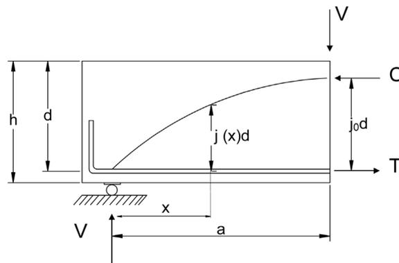
Fig. 2 Beam and arch actions
