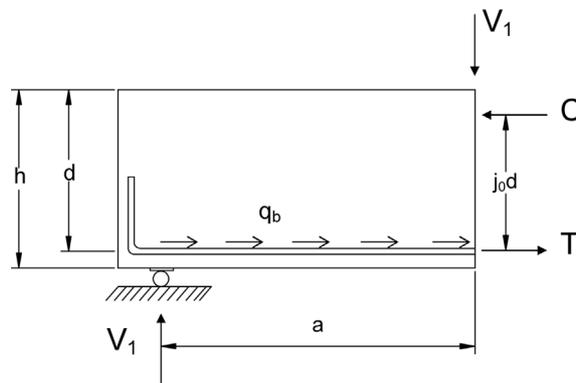
Fig. 3 Strength mechanism due to beam action
