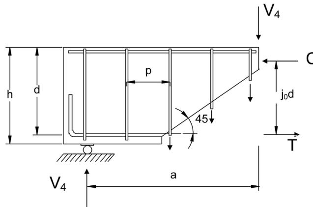
Fig. 9 Strength mechanisms due to stirrups across the principal crack
