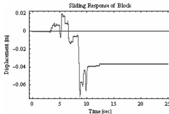
Fig. 4 Sliding of keel blocks in System I with ( $\mu_{s1} = 0.2, \mu_{s2} = 0.2$ )
