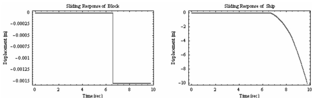
Fig. 19 Failure in System III due to extra sliding of the ship
