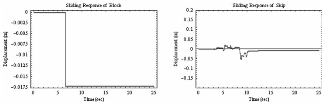
Fig. 11 Sliding of keel blocks and the ship in System 2 with ( $\mu_{s1} = 0.8, \mu_{s2} = 0.2$ )
