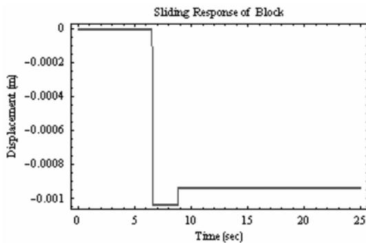
Fig. 13 Sliding of keel blocks in System I
