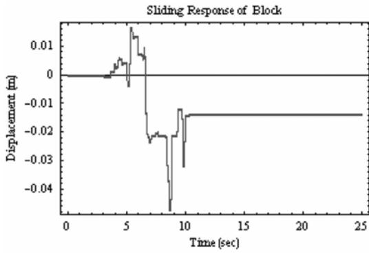
Fig. 15 Sliding of keel blocks in System I
