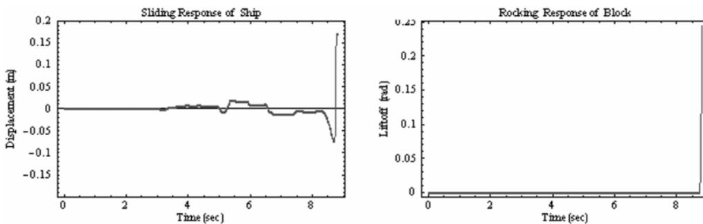
Fig. 6 Failure in System IV with  $(\mu_{s1} = 0.8, \mu_{s2} = 0.2)$  due to extra rocking of keel blocks
