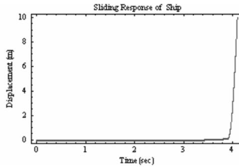
Fig. 17 Failure in System III due to extra sliding of the ship and keel blocks
