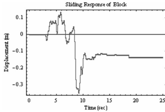
Fig. 8 Sliding of keel blocks in System I with  $(\mu_{s1} = 0.2, \mu_{s2} = 0.2)$
