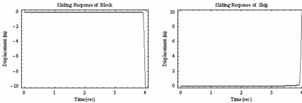
Fig. 9 Failure in System I with  $(\mu_{s1} = 0.8, \mu_{s2} = 0.2)$  due to extra sliding of keel blocks and the ship
