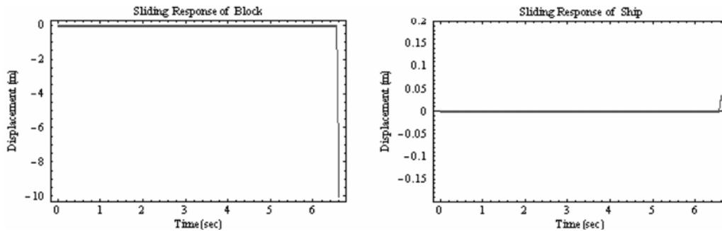
Fig. 5 Failure in System III with  $(\mu_{s1} = 0.5, \mu_{s2} = 0.5)$  due to extra sliding of keel blocks
