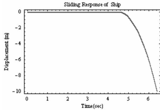
Fig. 16 Failure in System II due to extra sliding of the ship
