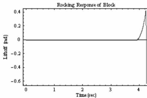
Fig. 18 Failure in System IV due to extra rocking of keel blocks
