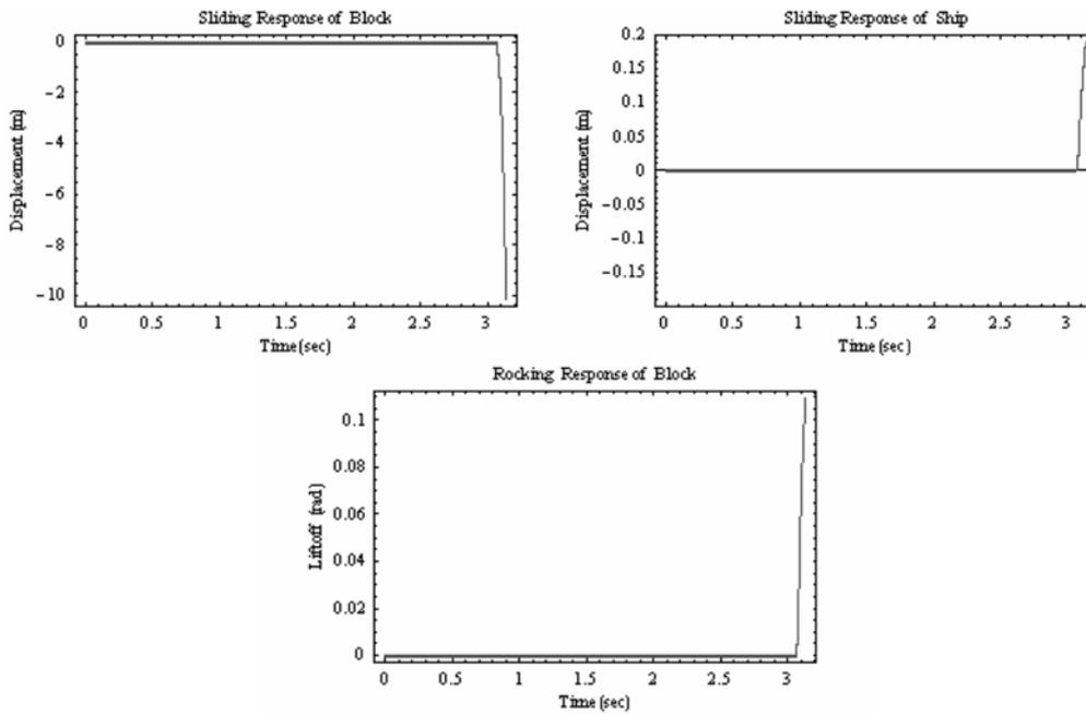
Fig. 10 Failure in System III with  $(\mu_{s1} = 0.5, \mu_{s2} = 0.5)$  due to extra sliding of keel blocks
