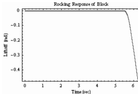
Fig. 12 Failure in System 3 with ( $\mu_{s1} = 0.8$ ,  $\mu_{s2} = 0.8$ ) due to extra rocking of keel blocks
