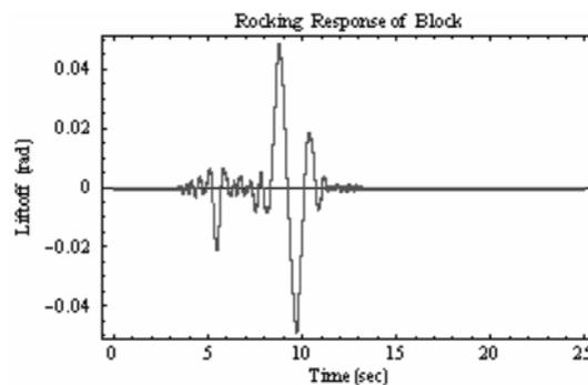
Fig. 7 Rocking of keel blocks in System IV with  $(\mu_{s1} = 0.8, \mu_{s2} = 0.8)$
