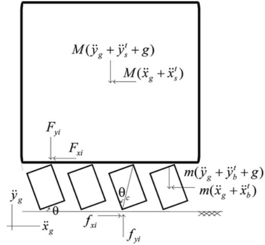
Fig. 5 Mode 3-Rocking of keel blocks around left bottom edge
