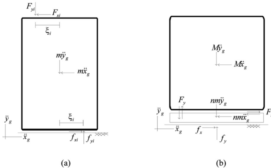
Fig. 3 Mode 1-Rest, (a) one keel block at rest, (b) the system at rest
