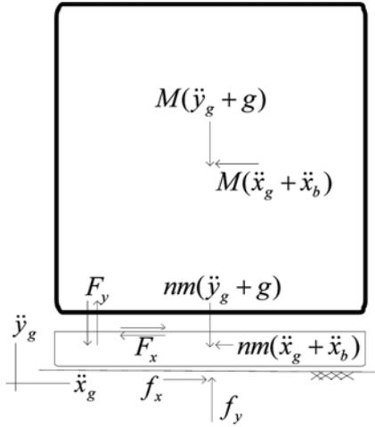
Fig. 4 Mode 2-Sliding of keel blocks
