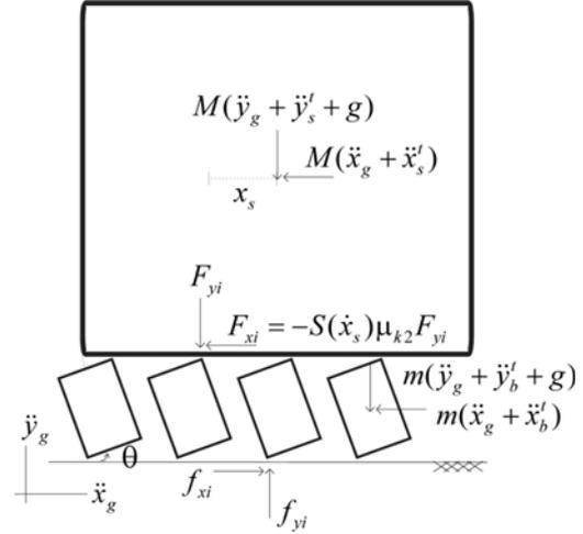
Fig. 9 Mode 7-Rocking of keel blocks with sliding of the ship
