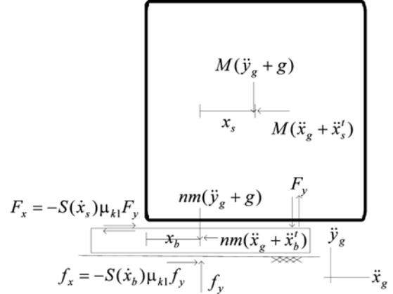
Fig. 7 Mode 5-Sliding of both keel blocks and the ship
