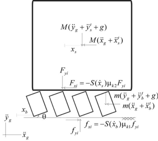
Fig. 10 Mode 8-Sliding and rocking of keel blocks accompanied with sliding of the ship
