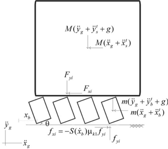
Fig. 8 Mode 6-Sliding and rocking of keel blocks
