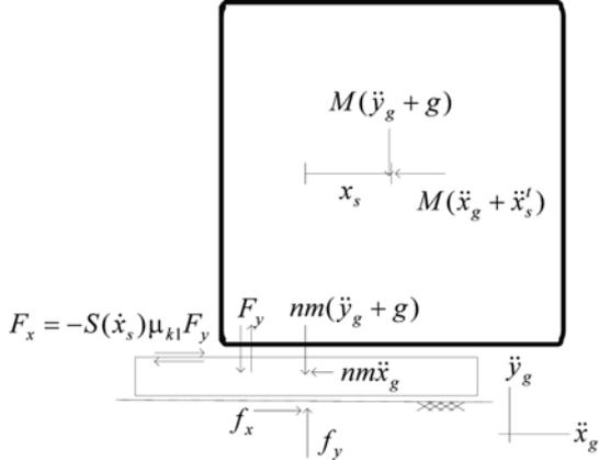
Fig. 6 Mode 4-Sliding of the ship
