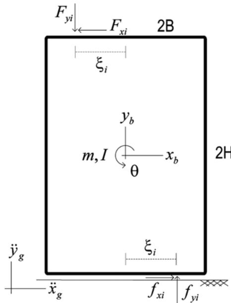
Fig. 2 Specifications of a sample block
