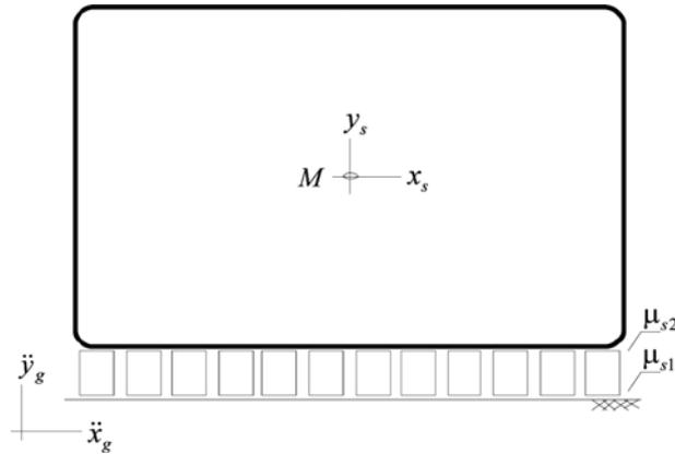
Fig. 1 A simple model of a ship over  $n$  similar keel blocks
