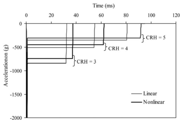
Fig. 7 Effect of CRH on deceleration of missile
