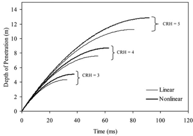
Fig. 6 Effect of CRH on penetration depth
