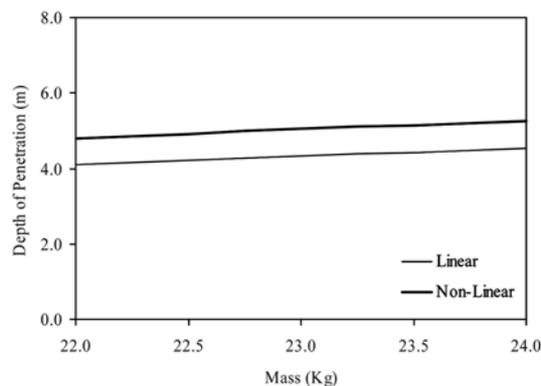
Fig. 9 Effect of missile mass on penetration depth
