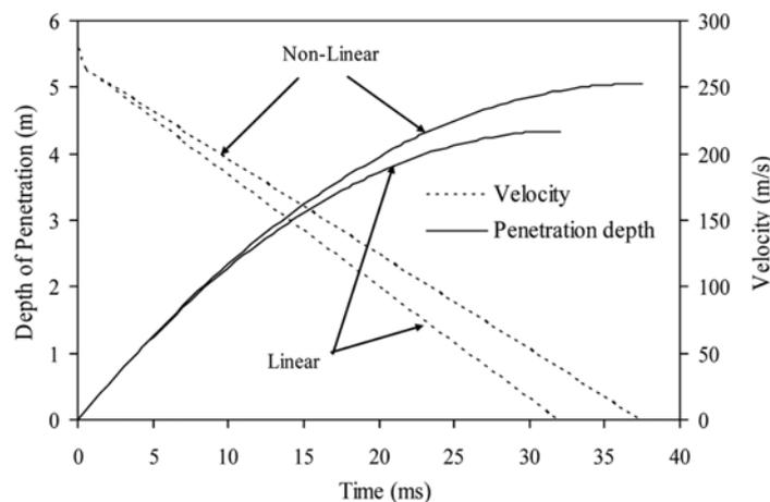
Fig. 5 Variation of penetration depth and velocity with time
