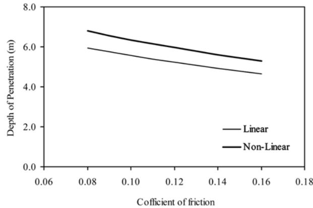
Fig. 8 Effect of coefficient of friction on penetration depth
