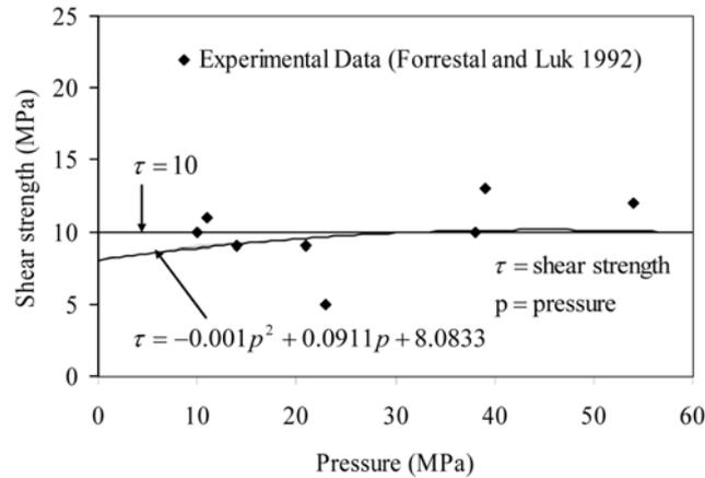
Fig. 3 Shear strength versus hydrostatic pressure for the soil target
