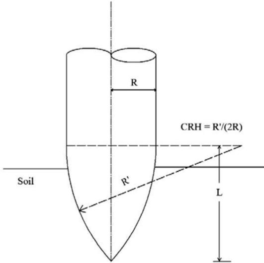
Fig. 1 A missile with ogival nose geometry
