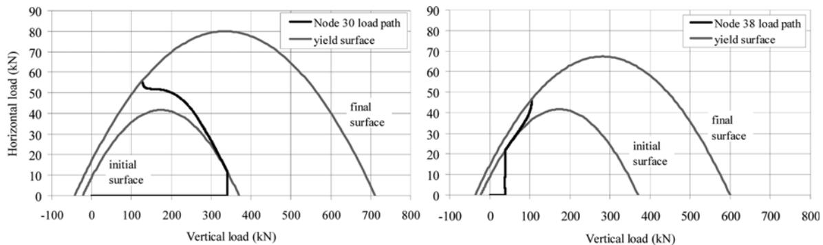
Fig. 4 Load paths of Node 30 and 38 showing the yield surface expansion
