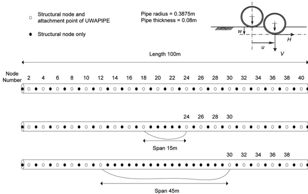
Fig. 1 Load and displacement sign convention and numerical model of pipeline system
