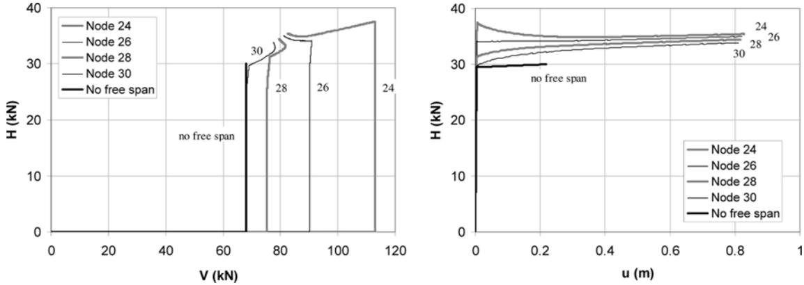
Fig. 2 Load and displacement for the no free span and 15 m span systems
