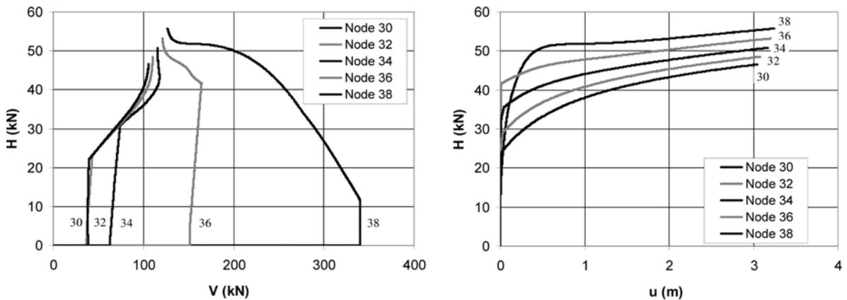
Fig. 3 Load and displacement for pipeline with a 45 m span
