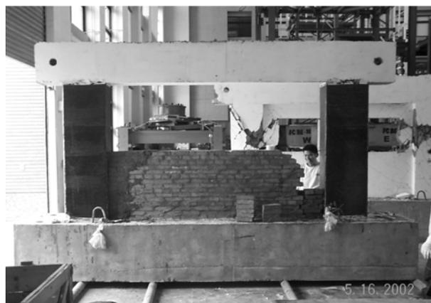
Fig. 3 Completion of brick wall (BMNFH10B-F)
