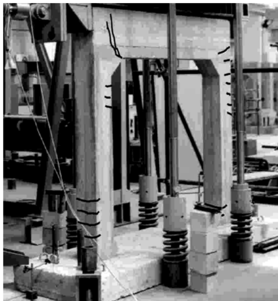
Fig. 8 Bare frame at the collapse: cracks distribution
