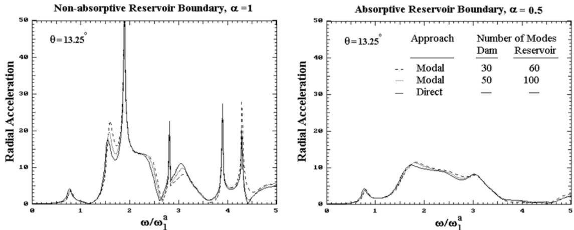
Fig. 5 Response at dam crest due to cross-stream ground motion
