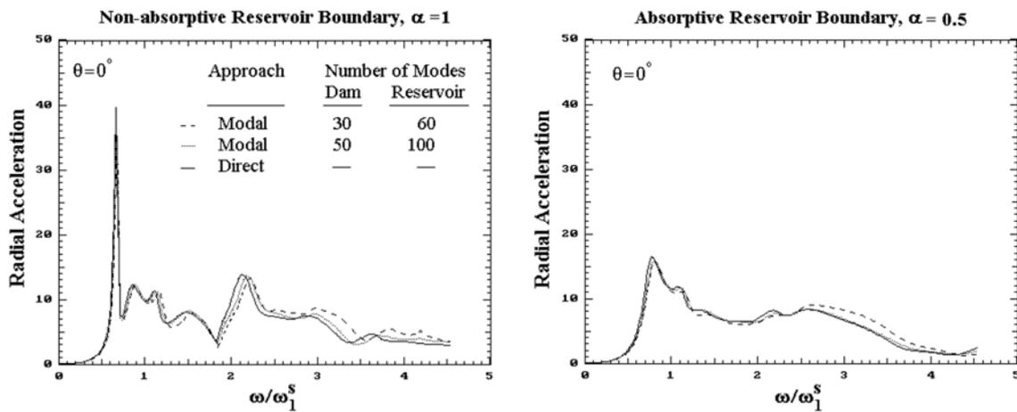
Fig. 3 Response at dam crest due to upstream ground motion
