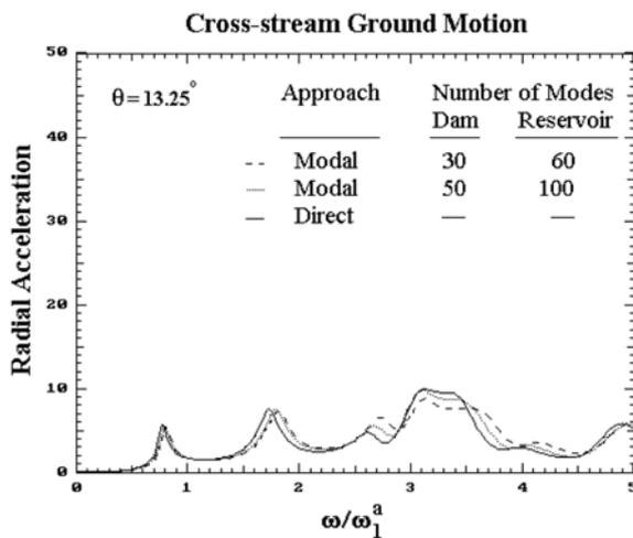
Fig. 8 Response at dam crest due to cross-stream excitation for the pseudo-incompressible condition
