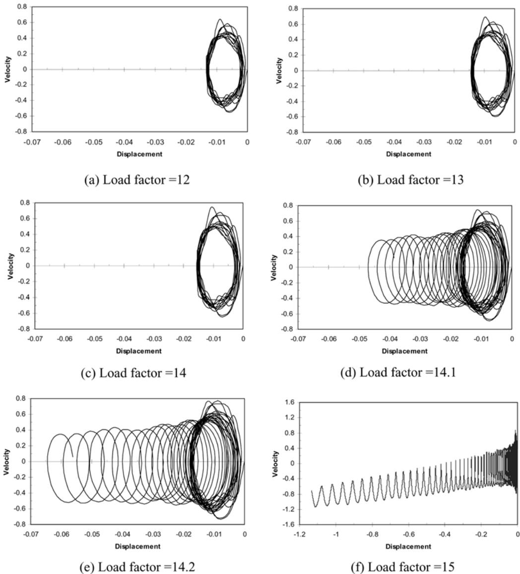
Fig. 6 Phase trajectory of square plate for different load factor values
