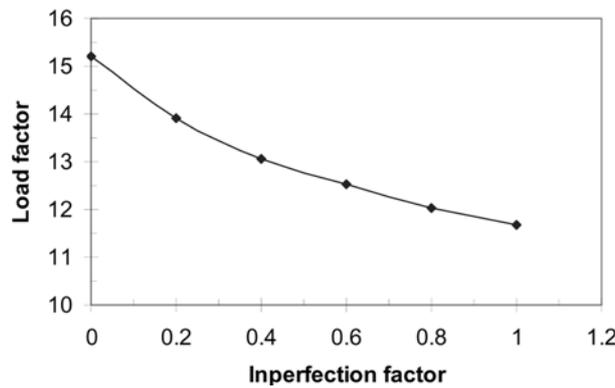
Fig. 5 Dynamic buckling load factors versus imperfection factors for square plate
