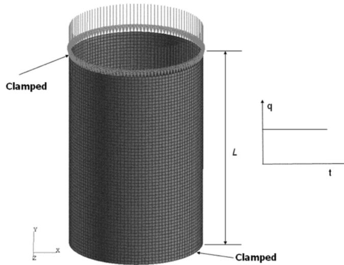
Fig. 7 Finite element mesh of a cylindrical shell subject to axial dynamic step load
