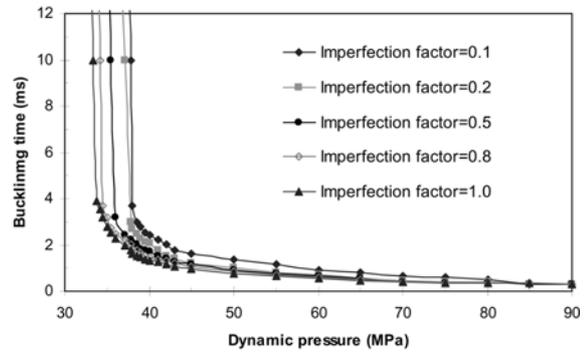
Fig. 16 Dynamic buckling time vs dynamic load pressure for cylindrical shell with different imperfection factors
