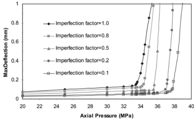
Fig. 9 Maximum transverse deflection of cylindrical vs dynamic axial pressure for respective imperfection factors
