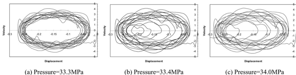
Fig. 14 Phase trajectory of cylindrical shell plate for different dynamic pressure values (Imperfection factor = 1.0)
