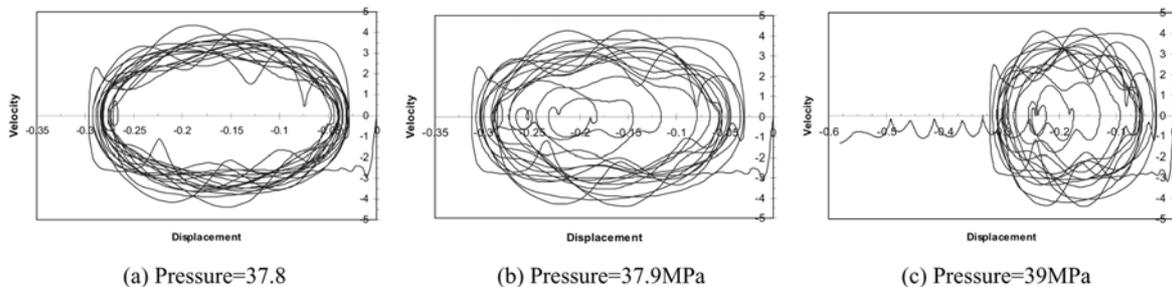
Fig. 10 Phase trajectory of cylindrical shell plate for different dynamic pressure values (Imperfection factor = 0.1)
