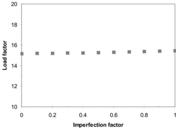
Fig. 3 Static buckling load factors vs imperfection factors
