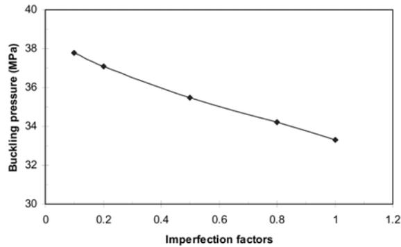
Fig. 15 Dynamic buckling pressure loads vs imperfection factors for cylindrical shell
