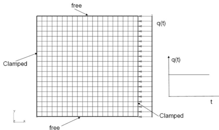
Fig. 1 The finite element mesh of a square plate and its loading
