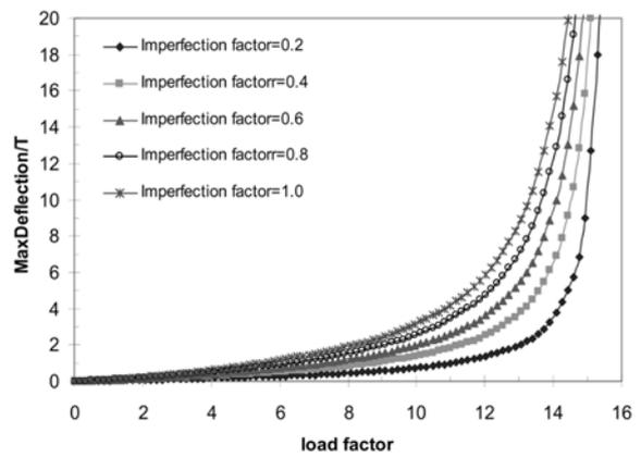
Fig. 4 Maximum transverse displacement of plate versus dynamic load factor with respective imperfection factors
