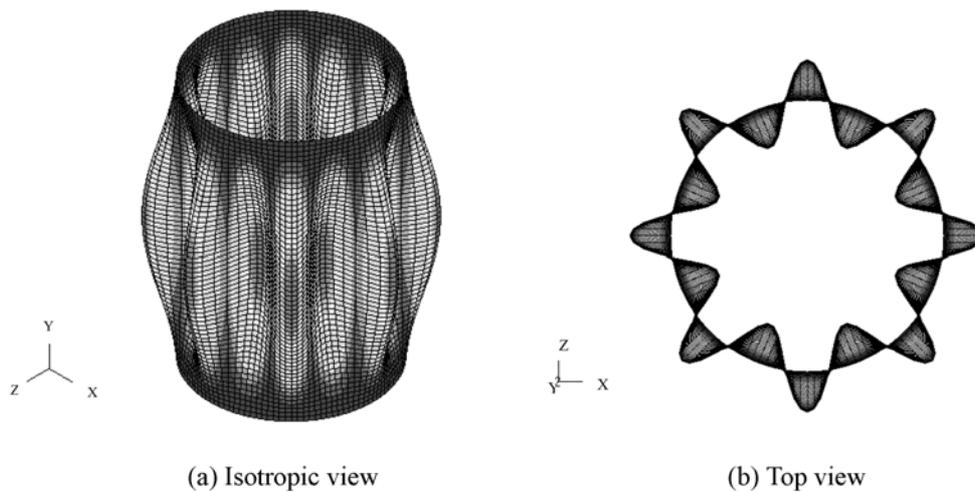
Fig. 8 First mode shape of clamped cylindrical shell
