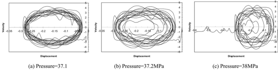
Fig. 11 Phase trajectory of cylindrical shell plate for different dynamic pressure values (Imperfection factor = 0.2)
