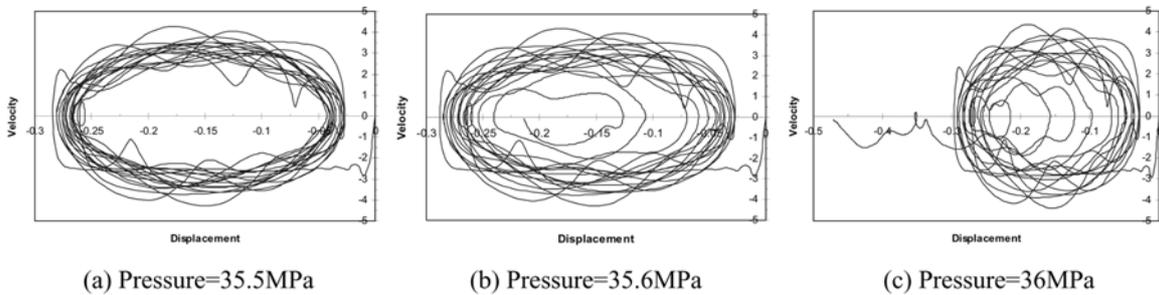
Fig. 12 Phase trajectory of cylindrical shell plate for different dynamic pressure values (Imperfection factor = 0.5)
