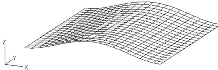
Fig. 2 First static buckling mode shape of a square plate
