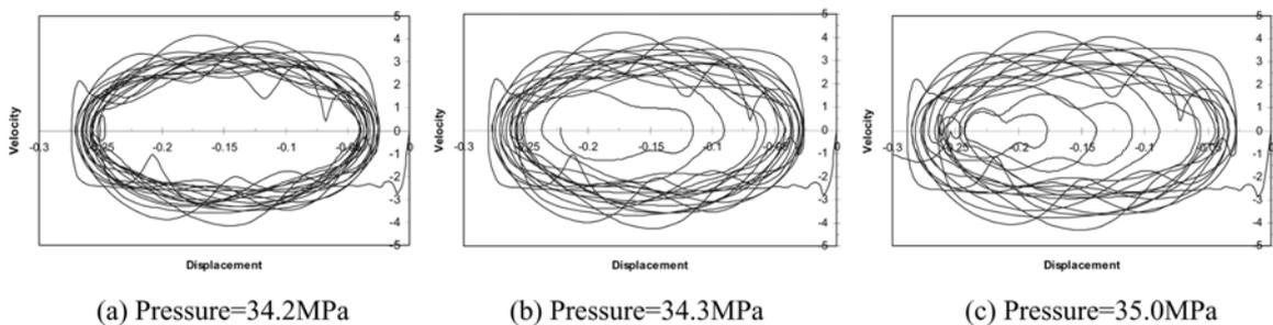
Fig. 13 Phase trajectory of cylindrical shell plate for different dynamic pressure values (Imperfection factor = 0.8)
