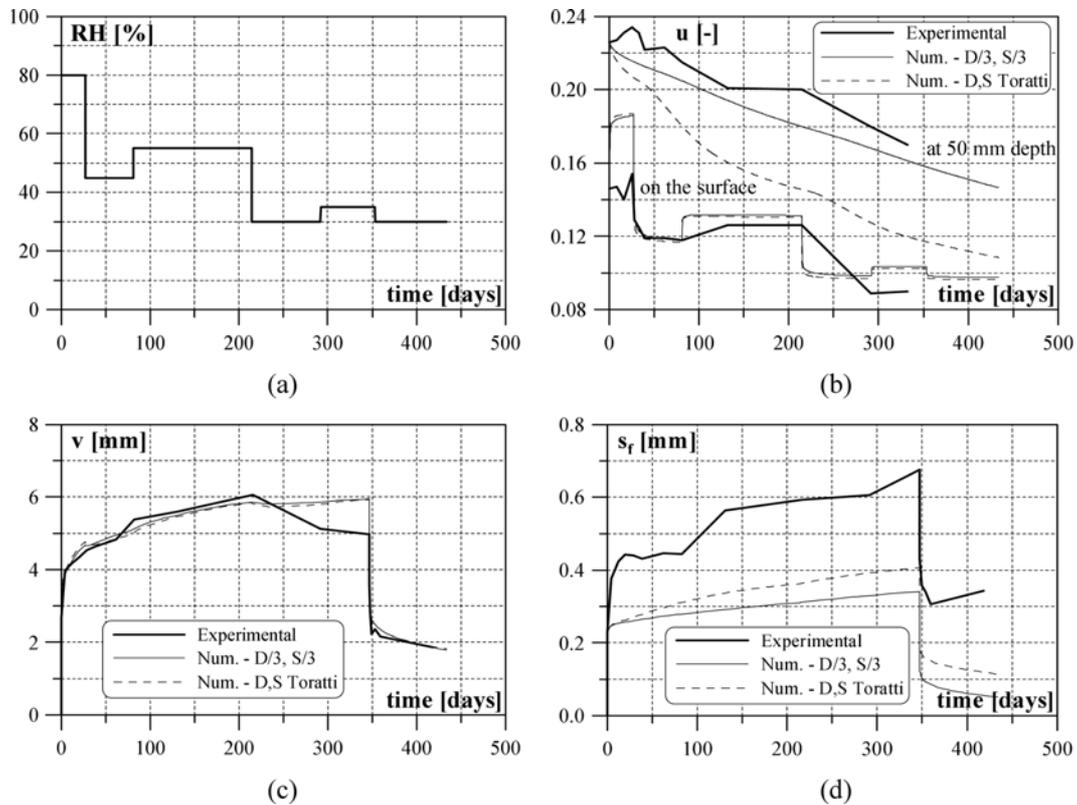
Fig. 5 Test performed by Bonamini *et al.* (1990): (a) relative humidity history of environment, (b) experimental-numerical comparisons in terms of timber moisture content on the surface and at 50 mm depth, (c) mid-span deflection and (d) slip over the supports
