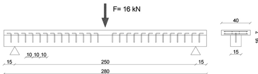
Fig. 4 Geometrical characteristics of the composite beam tested by Bonamini *et al.* (1990) (measures in cm)
