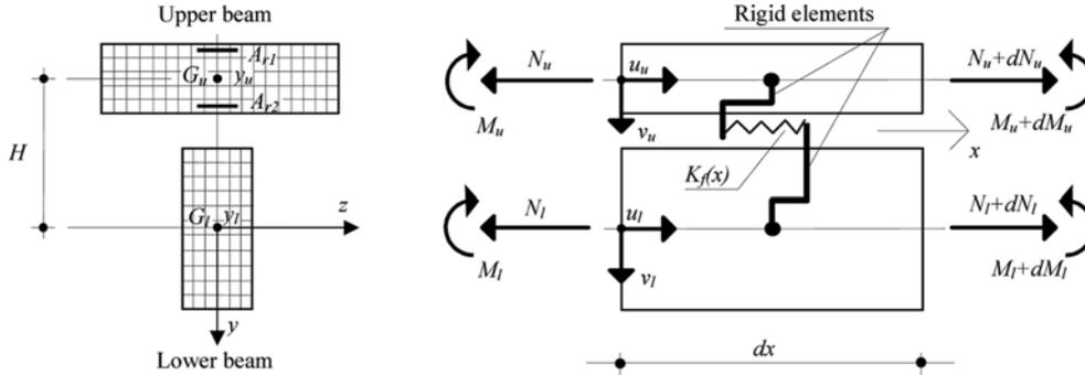
Fig. 1 The finite element used to model the composite beam
