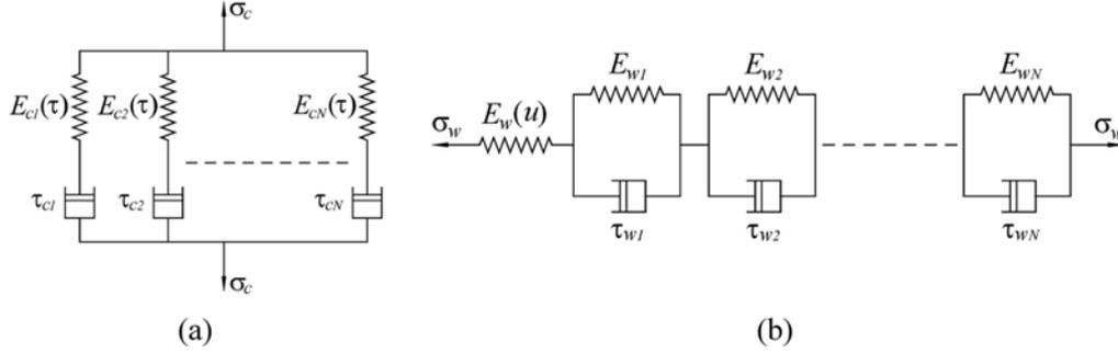
Fig. 2 (a) Maxwell's and (b) Kelvin's generalized rheological models used for concrete and timber, respectively
