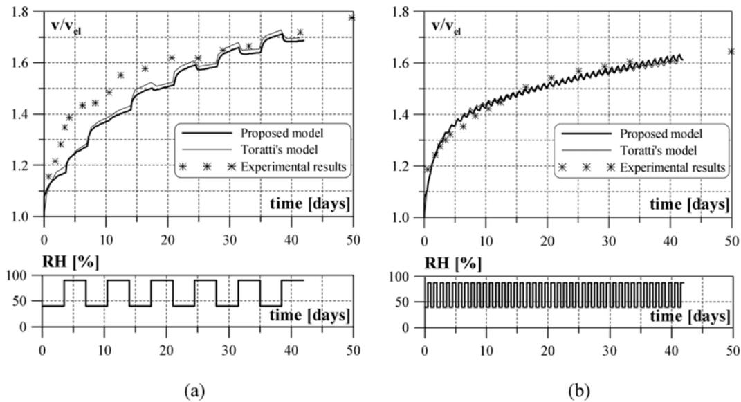
Fig. 3 Tests performed by Hoyle *et al.* (1986): (a) experimental-numerical comparison in terms of non-dimensional mid-span deflection on specimens subjected to weekly and (b) daily cycles of environmental relative humidity
