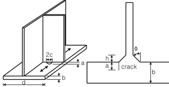
Fig. 7 Welding member of the bottom flange of a cross beam and vertical stiffener
