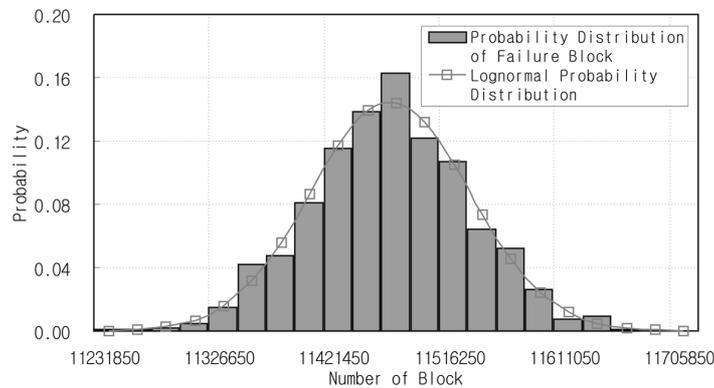
Fig. 8 Failure probability distribution of ADTT = 1000, Run = 1000
