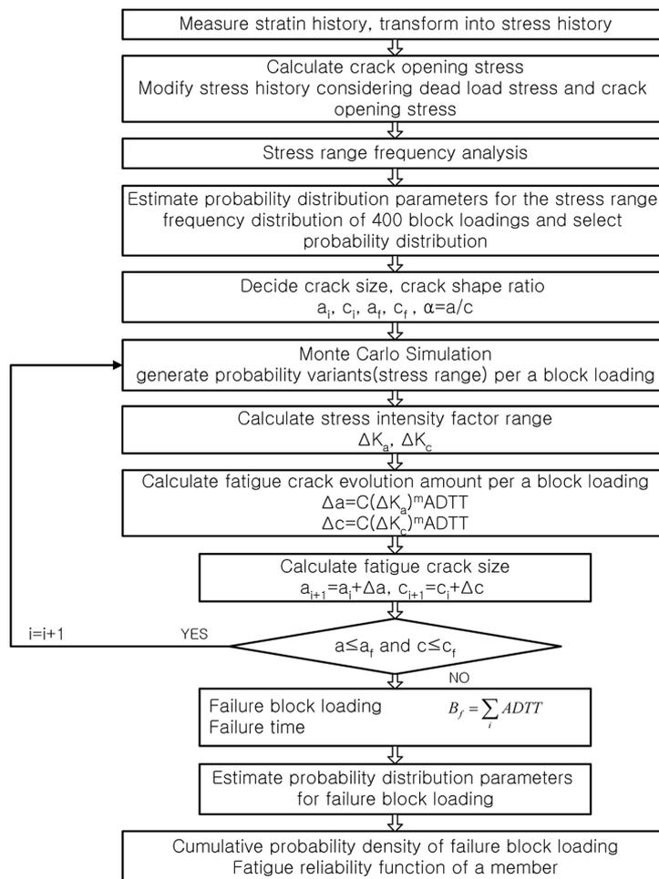
Fig. 3 Procedure of fatigue reliability analysis of a member
