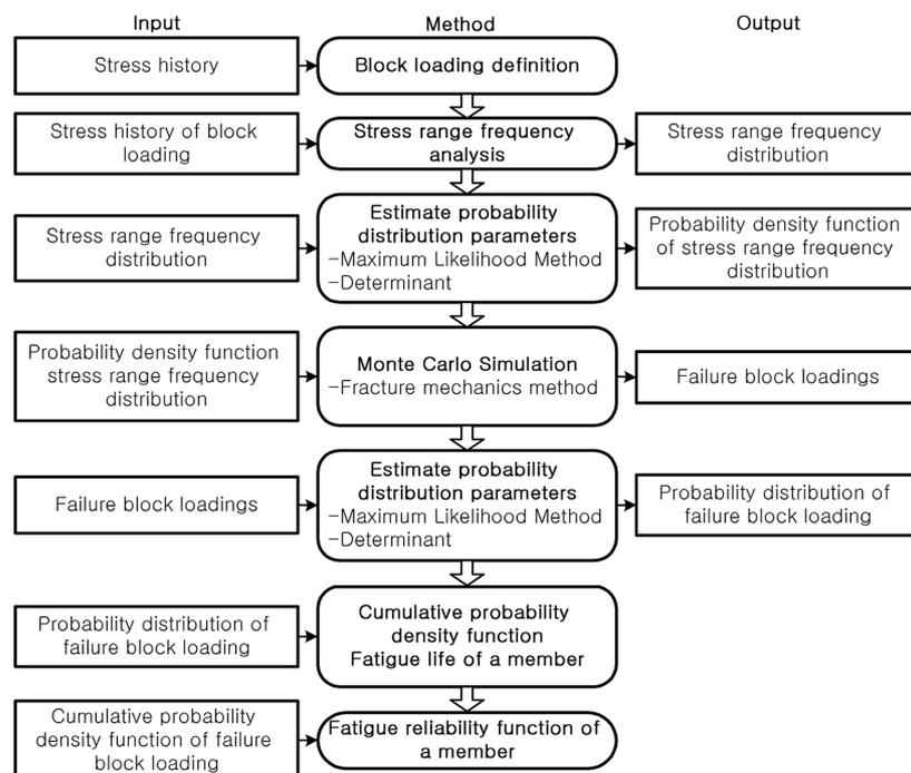
Fig. 1 Procedure of fatigue reliability analysis model
