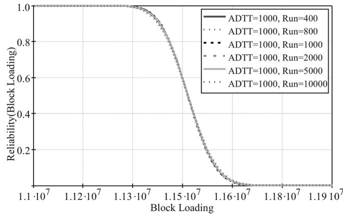
Fig. 9 Fatigue reliability according to simulations
