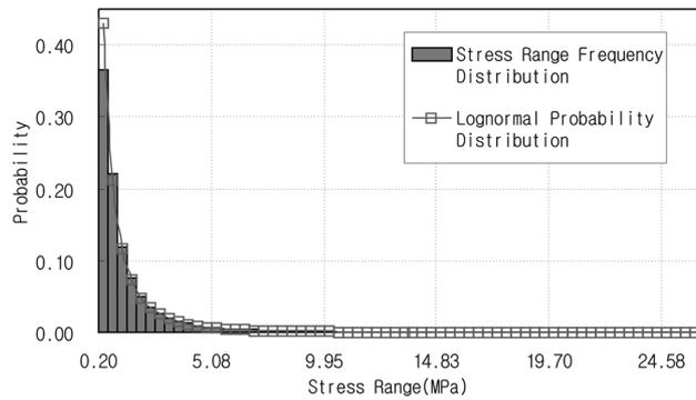
Fig. 6 Stress range frequency distribution & lognormal probability density for 400 block loadings
