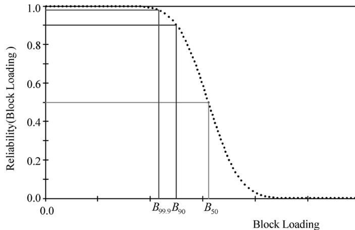
Fig. 2 Fatigue reliability function
