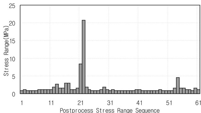
Fig. 5 Stress range considering loading sequence of a block loading
