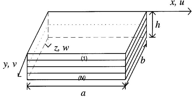
Fig. 1 Nomenclature of a laminated rectangular plate
