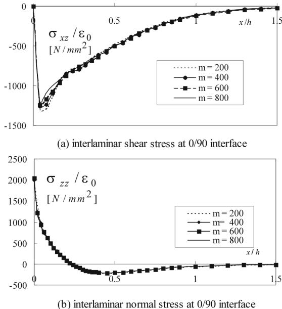
Fig. 2 Convergence of interlaminar stresses for [0/90]<sub>s</sub> laminate against different  $m$  with  $N=40$
