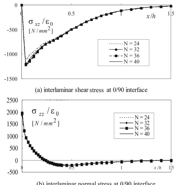
Fig. 3 Convergence of interlaminar stresses for [0/90]<sub>s</sub> laminate against different  $N$  with  $m=600$
