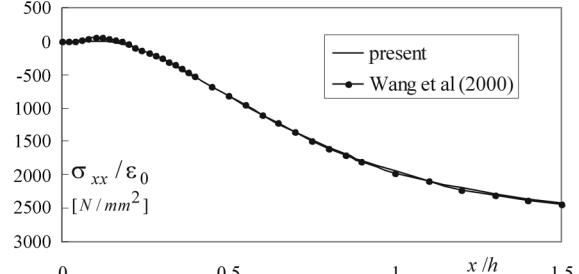
(b) in-plane stress at the middle interface of the laminate
