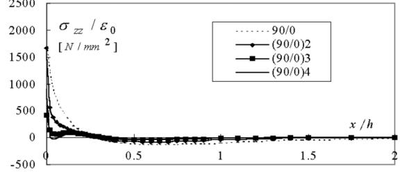
(a) interlaminar normal stress at middle surface of the plate
