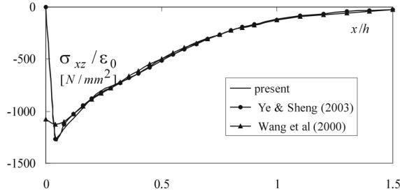
(a) interlaminar shear stress at the interface of [0/90]s
