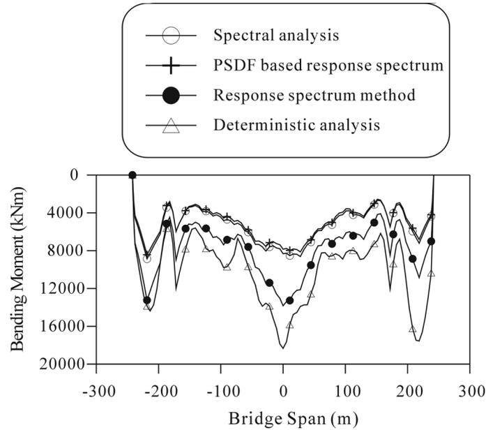
Fig. 8 Maximum deck bending moments for 600 m/s wave propagation velocity
