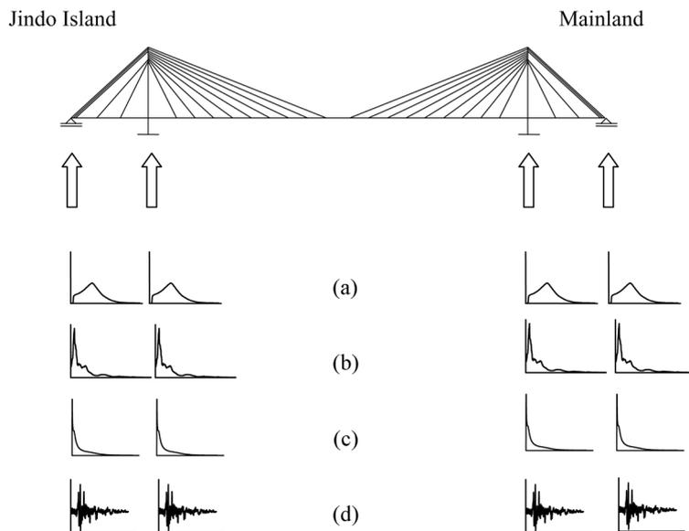
Fig. 4 Bridge model subjected to vertical ground motions (a) Spectral analysis, (b) Response spectrum method, (c) PSDF based response spectrum method, (d) Deterministic method
