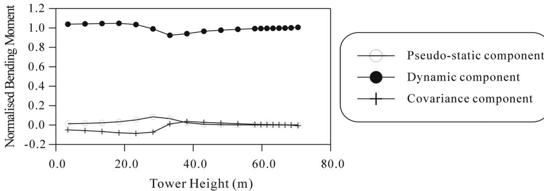
Fig. 16 Normalised bending moment variances of the island tower by response spectrum method
