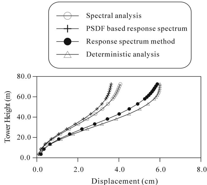
Fig. 7 Maximum horizontal displacements of the island tower for 600 m/s wave propagation velocity
