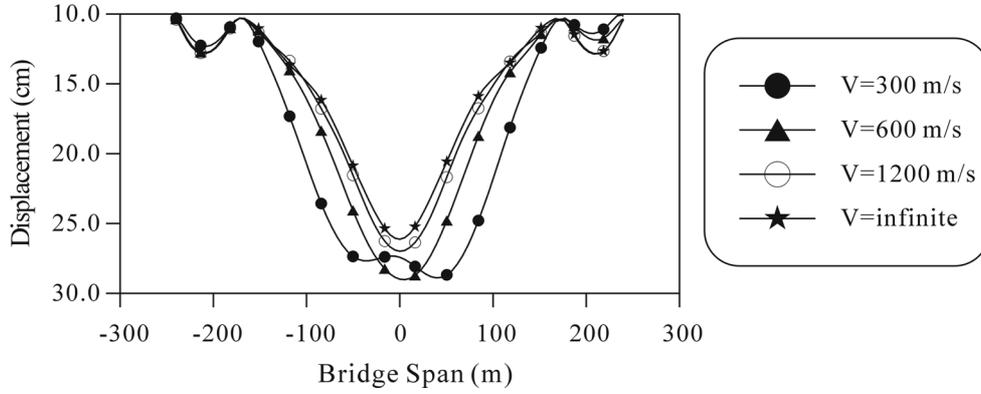
Fig. 9 Maximum vertical deck displacements by spectral analysis approach
