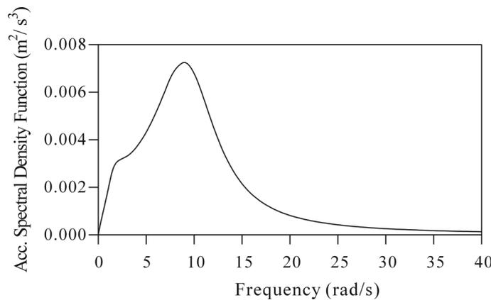
Fig. 1 Power spectral density function of ground motion for medium soil type
