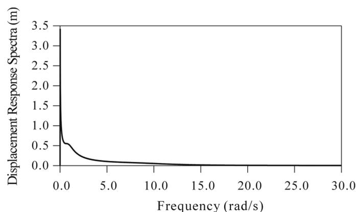
Fig. 5 Displacement response spectra obtained from Eq. (18) for medium soil type
