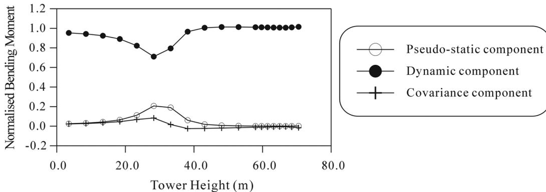
Fig. 15 Normalised bending moment variances of the island tower by spectral analysis approach
