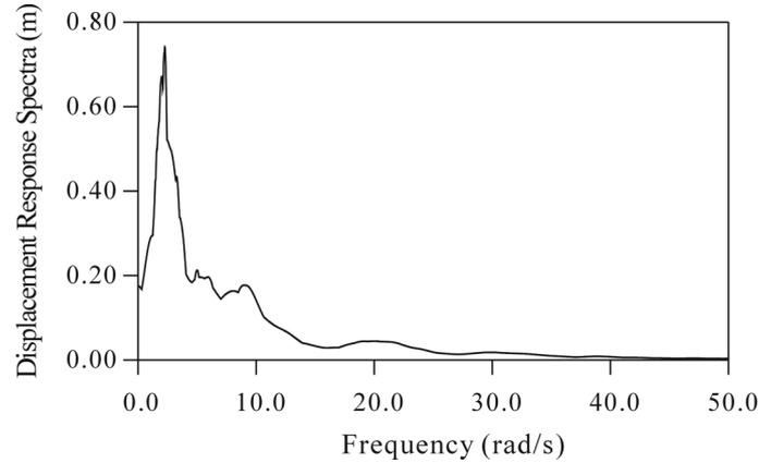
Fig. 2 Displacement response spectra for Erzincan earthquake
