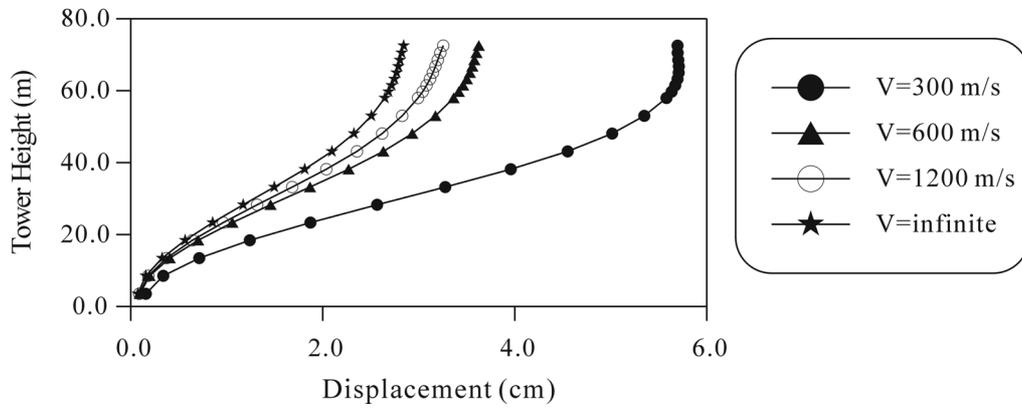
Fig. 12 Maximum horizontal displacements of the island tower by spectral analysis approach
