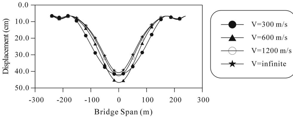
Fig. 10 Maximum vertical deck displacements by response spectrum method
