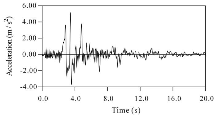
Fig. 3 Acceleration time history for east-west component of Erzincan earthquake
