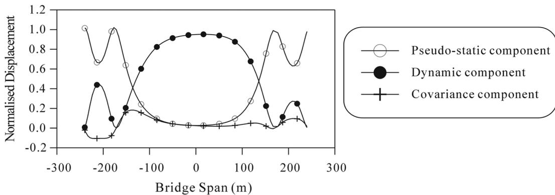
Fig. 14 Normalised displacement variances of the deck by response spectrum method
