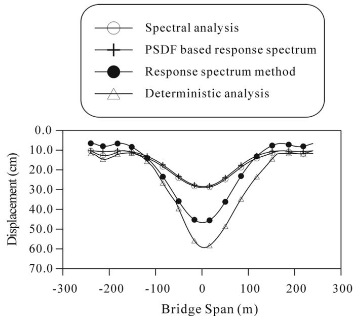
Fig. 6 Maximum vertical deck displacements for 600 m/s wave propagation velocity
