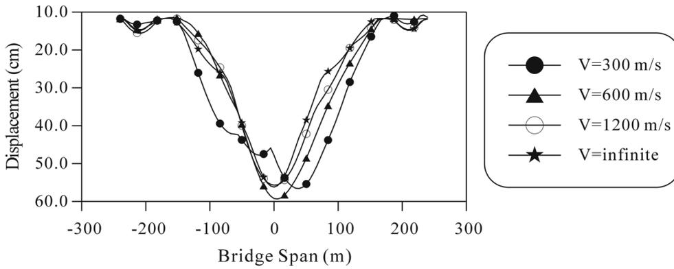
Fig. 11 Maximum vertical deck displacements by deterministic method
