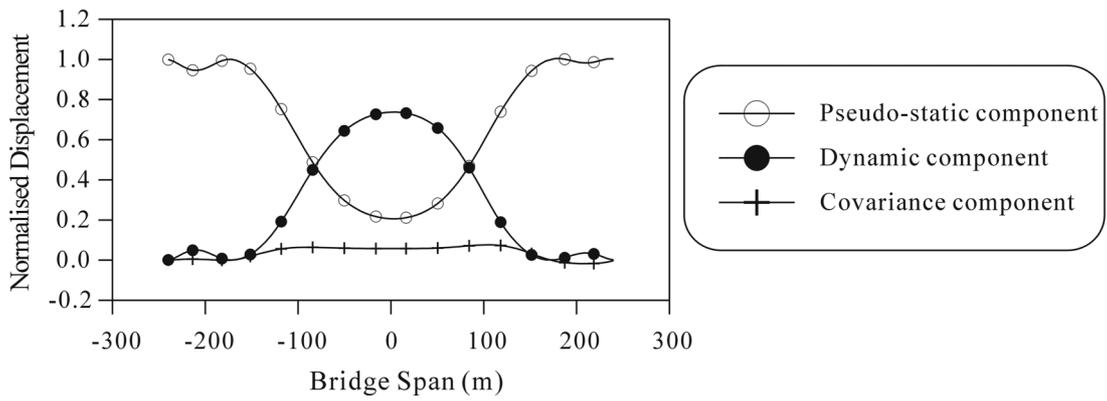
Fig. 13 Normalised displacement variances of the deck by spectral analysis approach
