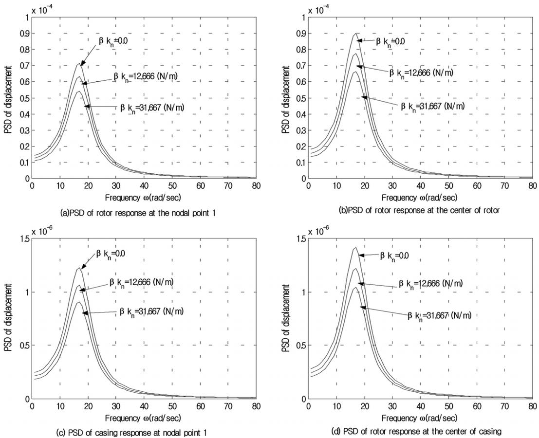
Fig. 6 Comparison of PSD of the response
