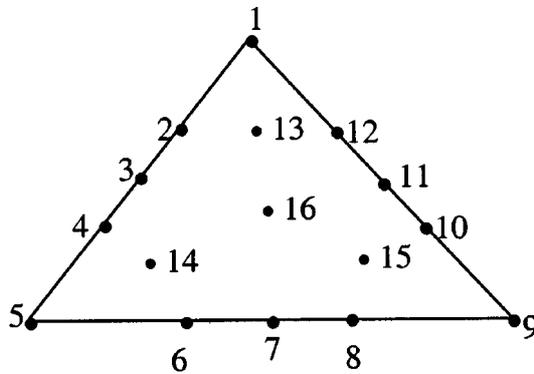
Fig. 1 A typical element with nodes
